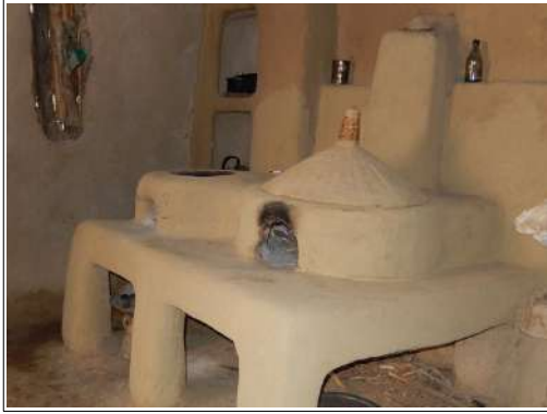
Picture 5: Improved injera baking stove. (Photo J. Boocock).
