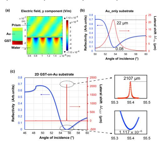
**Figure S2.** (a) Electric field distribution at SPR resonance angle 55.398°. (b) Simulation results of reflectivity and lateral position shift of Au-only substrate. (c) Simulation results of
