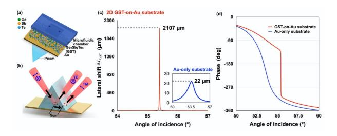
**Fig. 1** (a) Schematic of the sensing substrate based on GST-gold metastructures. (b) Schematic diagram of the giant lateral position shift induced by the GST-on-Au substrate. Simulation results of (c) lateral position shift and (d) optical phase signal change based on 2D GST-on-Au substrate and Au-only substrate.
