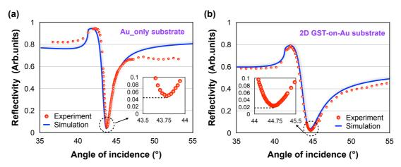
**Figure S4. Reflectivity spectra measurement.** (a) Au-only substrate (b) 2D GST-on-Au substrate.
