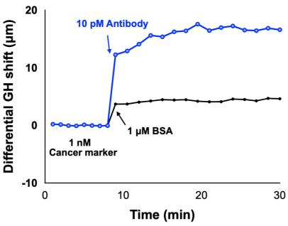
**Figure S7.** Detection of specific and non-specific binding based on lateral position shift. Blue curve shows the signal change when flowing capture antibody - monoclonal anti-TNF antibody to the sensing substrate while the black curve shows the signal change of flowing BSA as control antibody.
