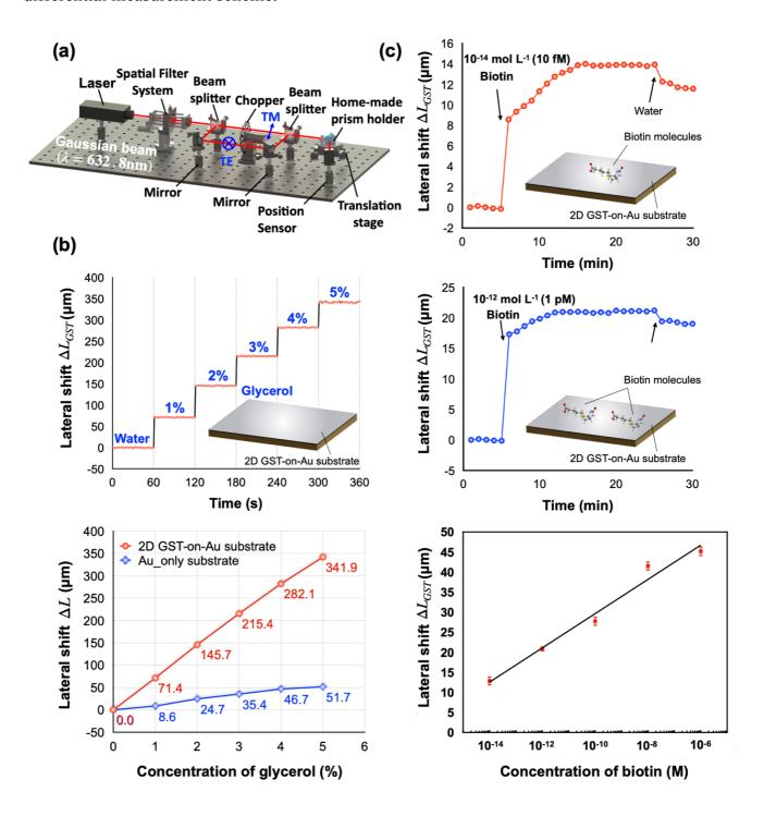
**Fig. 2** (a) Optical setup for measuring differential lateral position shift between *p*- and *s*-polarized light. (b) Evaluation results of measuring glycerol solutions. (c) Real-time detection of biotin molecules based on lateral position shift measurement.
