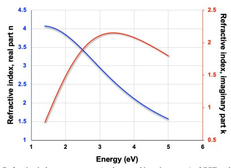
**Figure S3.** Refractive index measurement (real part and imaginary part) of GST under different photon energies.
