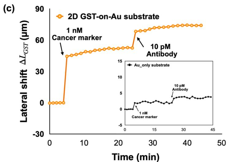
**Fig. 3** (a) Detection of extremely low (1 fM) cancer marker concentration using 2D GST-on-Au substrate. (b) Detection of 1nM cancer marker using 2D MoS<sub>2</sub>-on-Au substrate. (c) Detection of 1nM cancer marker using 2D GST-on-Au substrate with insert figure showing the performance of Au-only substrate.
