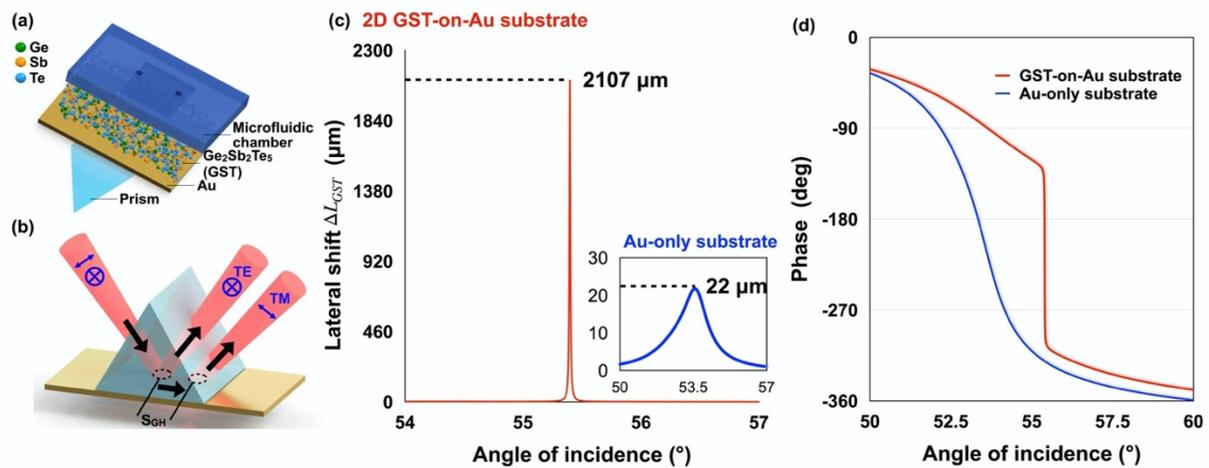
**Fig. 1** (a) Schematic of the sensing substrate based on GST-gold metastructures. (b) Schematic diagram of the giant lateral position shift induced by the GST-on-Au substrate. Simulation results of (c) lateral position shift and (d) optical phase signal change based on 2D GST-on-Au substrate and Au-only substrate.
