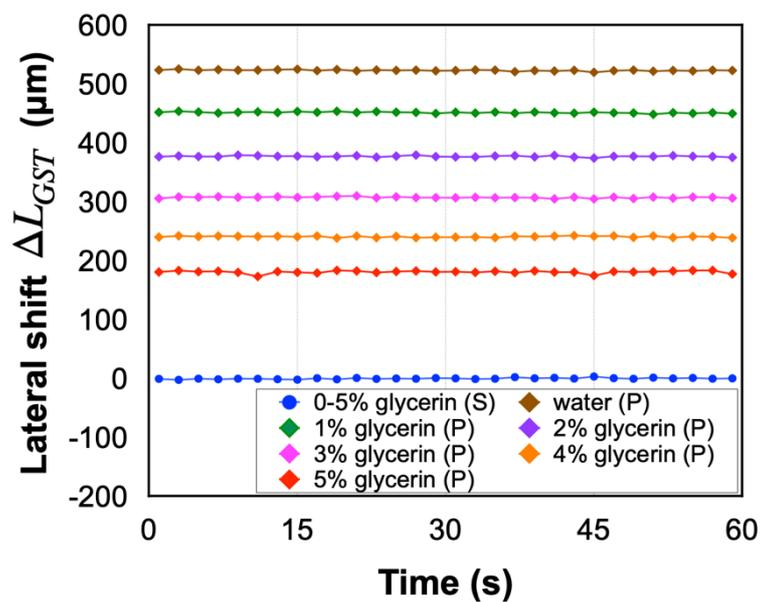
**Figure S5.** Lateral position shift of *p*-polarized and *s*-polarized light beam for different concentration levels of glycerol.
