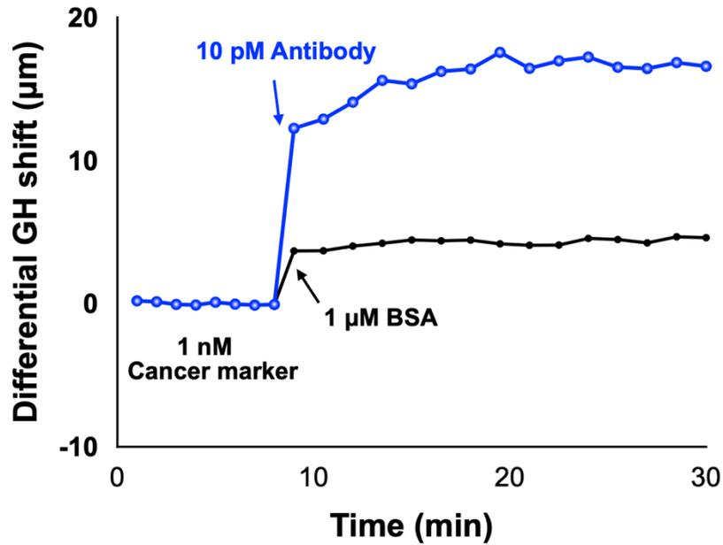
**Figure S7.** Detection of specific and non-specific binding based on lateral position shift. Blue curve shows the signal change when flowing capture antibody - monoclonal anti-TNF antibody to the sensing substrate while the black curve shows the signal change of flowing BSA as control antibody.
