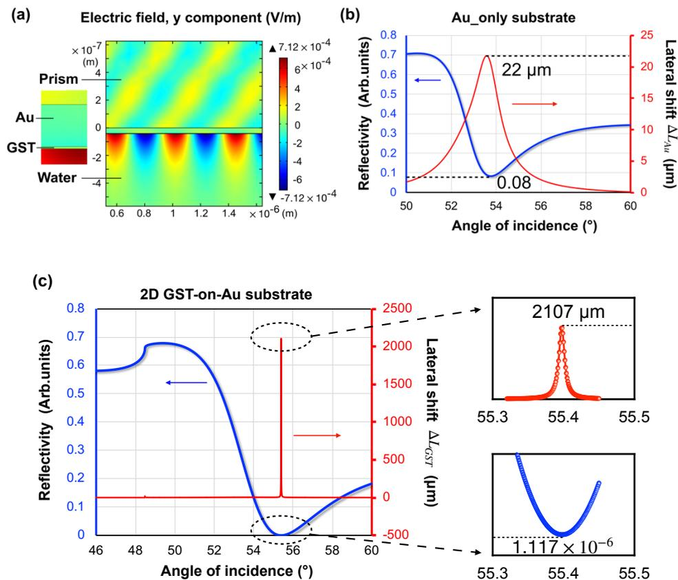
**Figure S2.** (a) Electric field distribution at SPR resonance angle  $55.398^\circ$ . (b) Simulation results of reflectivity and lateral position shift of Au-only substrate. (c) Simulation results of
