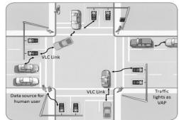
A communicating lighting system can reducing car roaming for parking. Locate a parking spot in a city is time consuming and polluting action. Smart lighting poles can locate available parking spots and broadcast information to driver's mobile phones or direct to smart cars.
