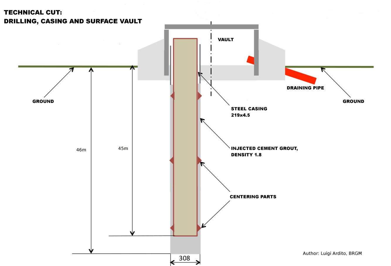
Scheme of the 45m deep posthole infrastructure, following the RESIF 5m deep posthole installation (Manhaval et al., 2015).
