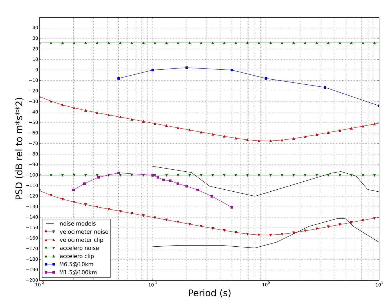
Technical characteristics of velocimetric sensor have been specified in order to measure a low noise for a M1.5 earthquake located 100 km away (Clinton et al. 2002). Therefore, in the case of such an event in Alsace, at least 4 stations would detect it.
