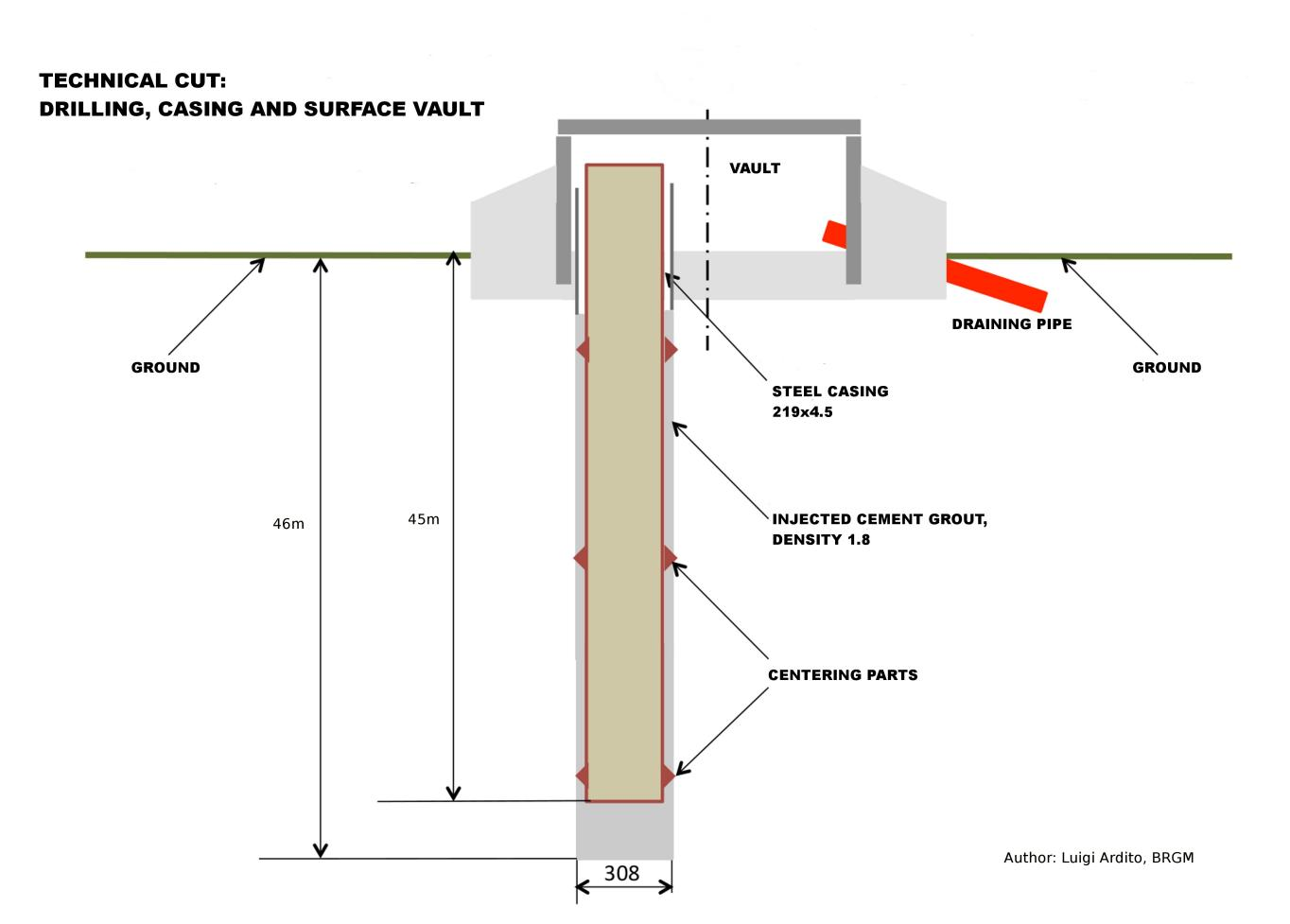
Scheme of the 45m deep posthole infrastructure, following the RESIF 5m deep posthole installation (Manhaval et al., 2015).
