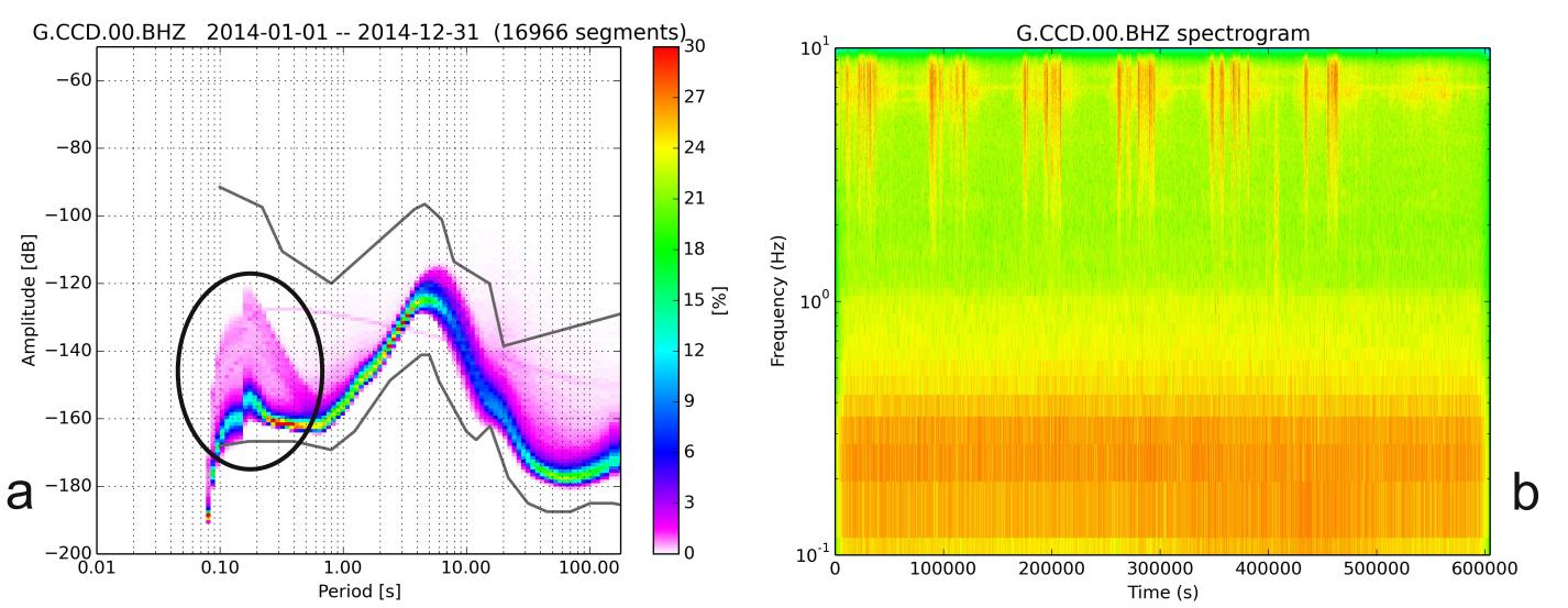
Probablity of Power Spectral Density (PPSD) over the year 2014 (a) and typical week spectrogram (b).
