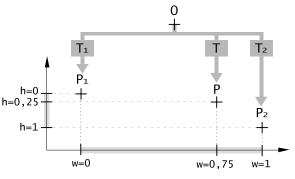
Figure 8: Geometrical interpretation of orthogonal interpolation. Here, an intermediate transformation T is applied to a point O, with  $T = I_{((0,0),T_1),((1,1),T_2)}^{orth}$  (0.75, 0.25).
