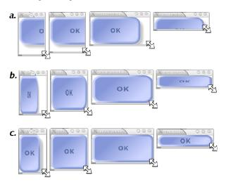
Figure 3: Three resizing strategies for a vector graphics button: fixed layout (a), naive scaling (b) and commonly expected resizing (c).
