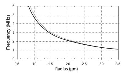
Figure 8.1: Resonance frequencies of free (bold line) and lipidencapsulated (thin line) air microbubbles in water as a function of equilibrium radius.
