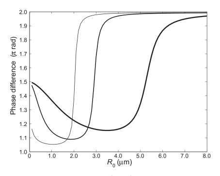
Figure 8.4: Phase angle difference  $(\phi + \pi)$  between a damped radially oscillating bubble and an incident 2-MHz sound field, as a function of equilibrium radius  $R_0$ . The thin line represents a free bubble, the medium line a SonoVue<sup>TM</sup> microbubble, and the thickest line an Albunex<sup>(R)</sup> microbubble.
