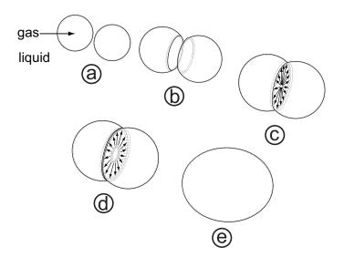
Figure 8.8: Schematic representation of stages of expanding bubble coalescence: (a) bubble collision, (b) flattening of contact surfaces, (c) liquid film drainage until a critical thickness (d), (e) film rupture, and (f) formation of an ellipsoidal bubble.
