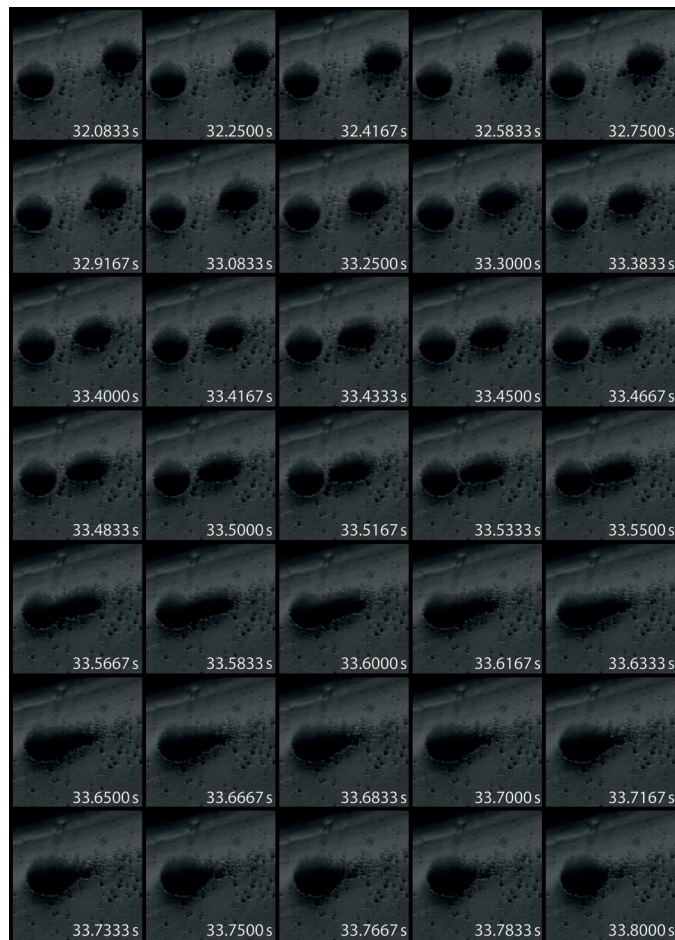
Figure 15 – Two clusters, with 22- \mu\text{m} diameters and an initial distance of 55- \mu\text{m} , colliding and merging during continuous sonication at a 2-MHz driving frequency and a 20-kPa peak-negative pressure. The frame size corresponds to 81 \times 81 (\mu\text{m})^2 . Times are relative to the start of the sonication ( t = 0 ).
