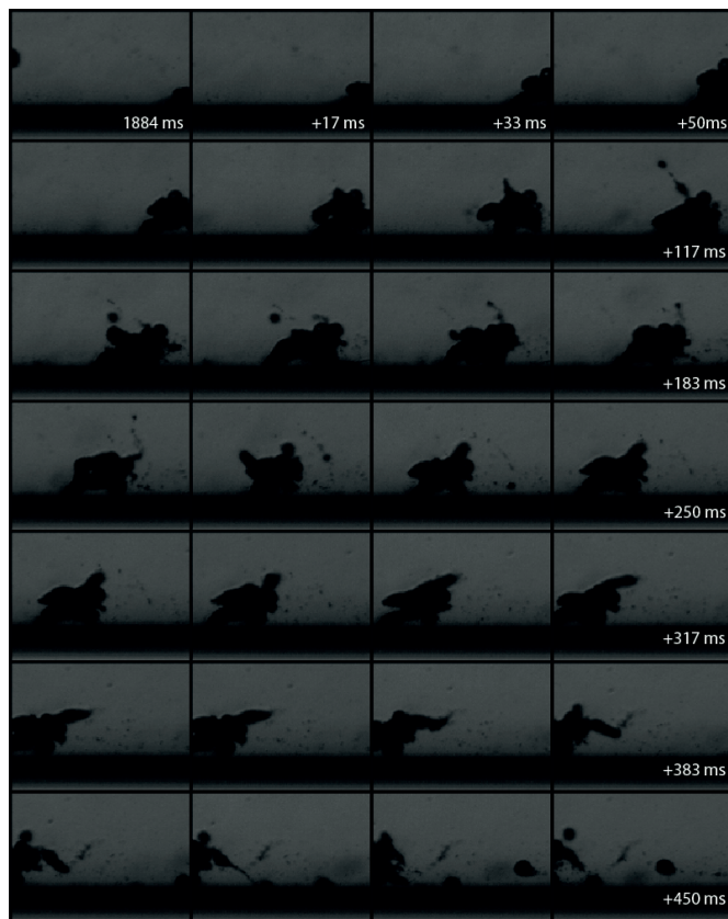
Figure 18 - Morphing microfoam during sonication at 7 MHz and 86 kPa peak-negative pressure and a schematic representation of the event. The frame size corresponds to 274 \times 198 (\mu\text{m})^2 . Time t = 0 was defined by the start of the sonication.
