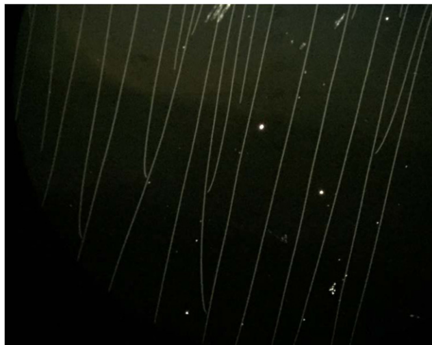
Figure 21. Cracks observed on an IBS \text{Ta}_2\text{O}_5\text{-ZrO}_2 thin film (LMA) after annealing at T_a = 700^\circ\text{C} .
