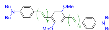
6a n = 1 , \sigma_{2PA} = 900 GM at 730 nm (ns-TPEF) 6b n = 2 , \sigma_{2PA} = 1250 GM at 775 nm (ns-TPEF)
