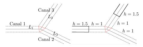
FIGURE 12. On the left the 2D numerical domain for the comparison with the 1D geometry. On the right the 2D initial water height in a merging junction.
