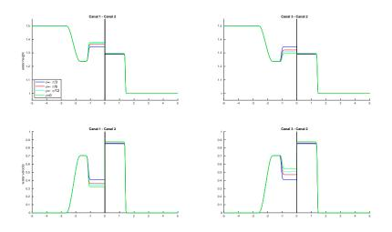
FIGURE 11. Test 5.3: comparison of the solution for various geometries in the case of a merging at T = 0.5,  $s_1 = s_2 = s_3 = 1$ ,  $\theta = \pi/3$  and  $\phi = -\pi/3, -\pi/6, -\pi/12, 0$ . On the left: zoom on the transition between canal 1 and 2; on the right: zoom on the transition between canal 3 and 2. Initial data are given at Eq.(39).
