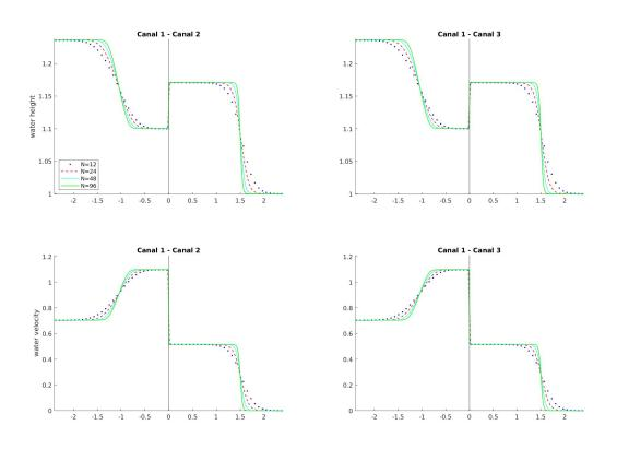
FIGURE 7. Test 5.1: numerical convergence at time T = 0.9, after the shock has reached the junction. N = 12, 24, 48, 96. On top: water height as a function of x; on bottom: water velocity as a function of x. On the left: canal 1 and 2; on the right: canal 1 and 3. Initial data are given in (38).
