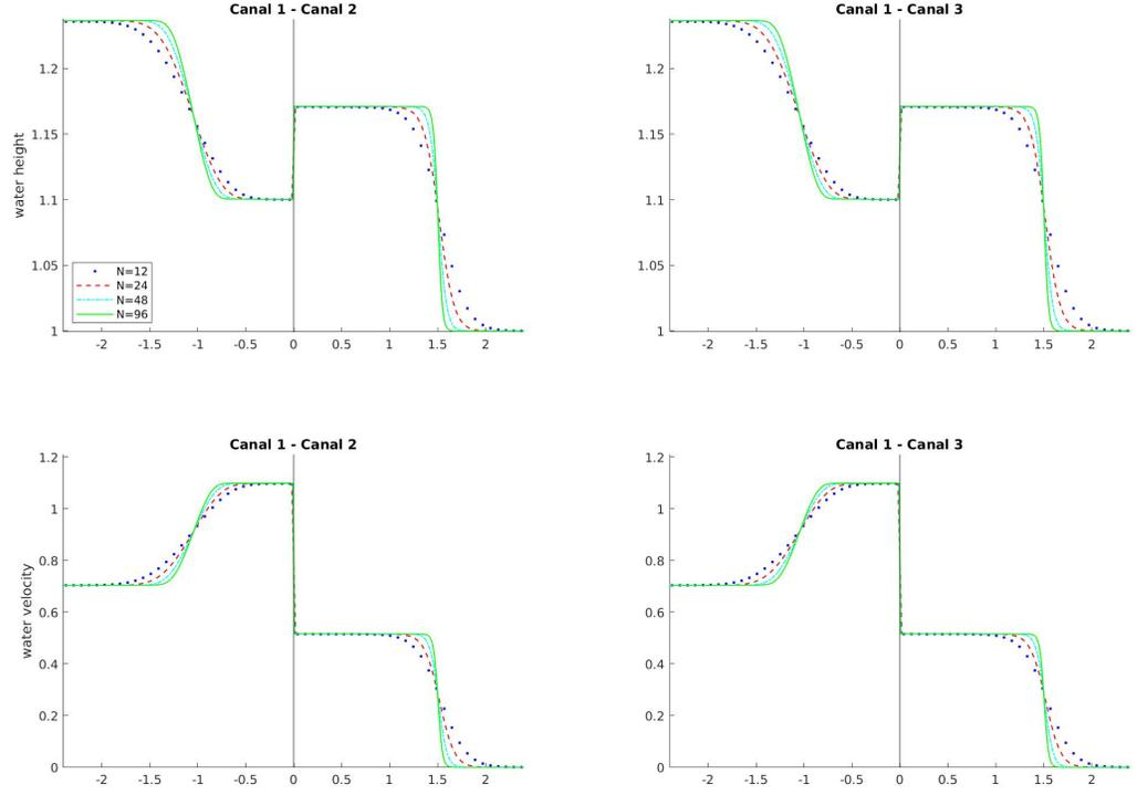
FIGURE 7. Test 5.1: numerical convergence at time  $T = 0.9$ , after the shock has reached the junction.  $N = 12, 24, 48, 96$ . On top: water height as a function of  $x$ ; on bottom: water velocity as a function of  $x$ . On the left: canal 1 and 2; on the right: canal 1 and 3. Initial data are given in (38).
