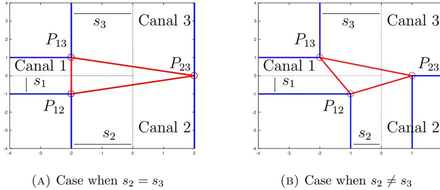
FIGURE 5. Junction - Particular case of the T-junction. Parameters are  $\theta = -\phi = \frac{\pi}{2}$  and  $s_1 = 1$ ,  $s_2 = s_3 = 2$  (on the left) and  $s_1 = s_2 = 1$ ,  $s_3 = 2$  (on the right).
