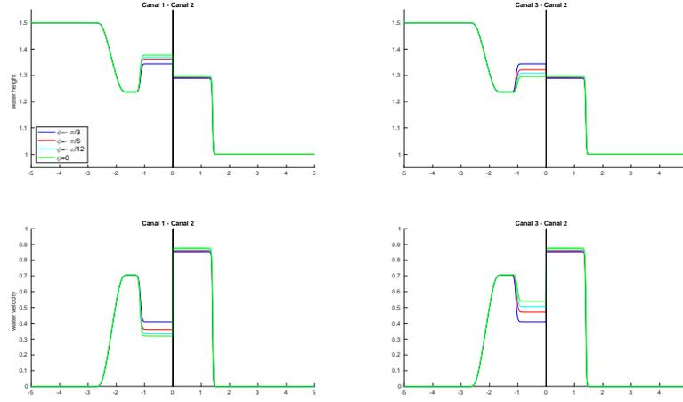
FIGURE 11. Test 5.3: comparison of the solution for various geometries in the case of a merging at  $T = 0.5$ ,  $s_1 = s_2 = s_3 = 1$ ,  $\theta = \pi/3$  and  $\phi = -\pi/3, -\pi/6, -\pi/12, 0$ . On the left: zoom on the transition between canal 1 and 2; on the right: zoom on the transition between canal 3 and 2. Initial data are given at Eq.(39).
