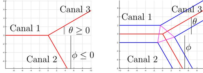
FIGURE 1. A 3 canal junction. On the left, the 1D set-up; on the right, the 2D configuration.
