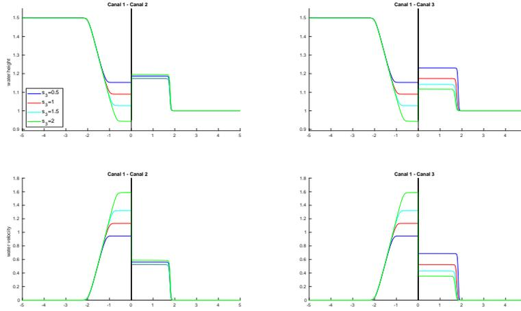
FIGURE 10. Test 5.2: comparison of various geometries with different sections at  $T = 0.5$ .  $\theta = -\phi = \pi/4$ ,  $s_1 = s_2 = 1$  and  $s_3 = 0.5, 1, 1.5, 2$ . On the left: zoom on the transition between canal 1 and 2; on the right: zoom on the transition between canal 1 and 3. Initial data are given at Eq.(38).
