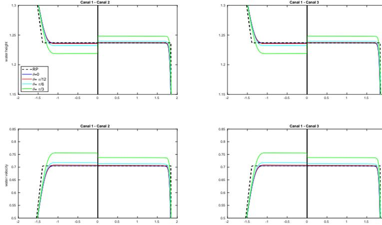
FIGURE 8. Test 5.2: comparison of various symmetric geometries with the solution on a single canal at  $T = 0.5$ :  $s_1 = 1$  and  $s_2 = s_3 = 1/2$ ;  $\phi = -\theta$  and  $\theta = 0, \pi/12, \pi/6, \pi/3$ . Black dashed line: 1D exact shallow-water on a single channel; Blue solid line: numerical solution for  $\theta = \phi = 0$ . On the left: zoom on the transition between canal 1 and 2; on the right: zoom on the transition between canal 1 and 3. Initial data are given in (38).
