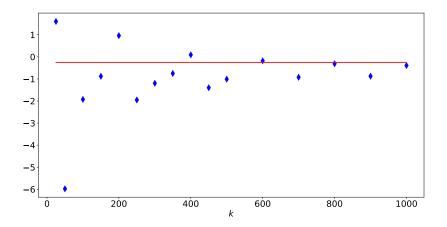
Figure 15: Determination of  $\partial_x \partial_y f_r(0)$  for the spin-oscillator using Formula (56) with x = 0.01 and  $\lambda = 1$ , for different values of k. The red line corresponds to the theoretical result  $\partial_x \partial_y f_r(0) = -\frac{1}{4}$ .
