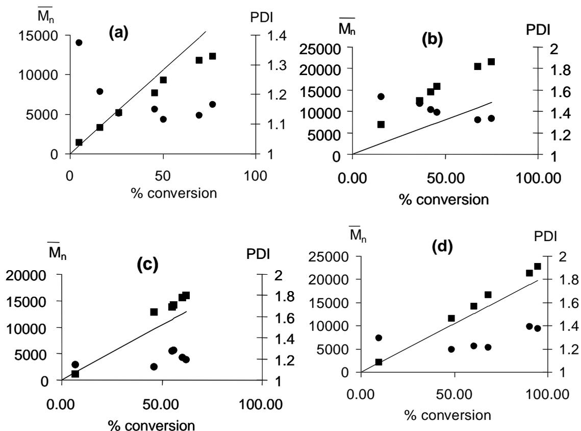
**Figure 6.**  $\bar{M}_n$  vs. conversion and PDI for the ATRP of styrene catalyzed by  $\text{MoOX}_2(\text{PMe}_3)_3$  (X = Cl, I). The conditions are given in Table 3 (entries 1-4). Squares: experimental  $\bar{M}_n$ ; circles: PDI; straight line: theoretical  $\bar{M}_n$ . (a) X = Cl, no Al(OiPr)<sub>3</sub> (entry 1); (b) X = Cl, with Al(OiPr)<sub>3</sub> (entry 2); (c) X = I, no Al(OiPr)<sub>3</sub> (entry 3); (d) X = I, with Al(OiPr)<sub>3</sub> (entry 4).
