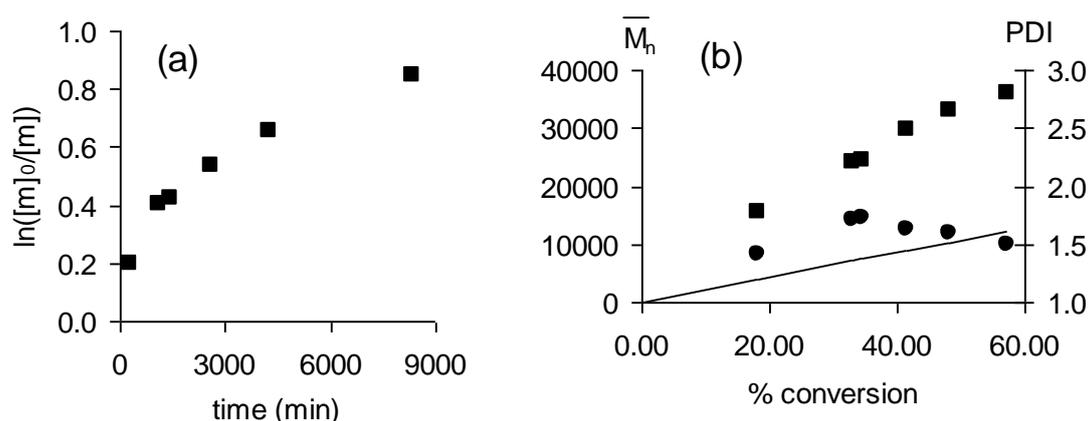
**Figure 7.** Polymerization of methyl acrylate catalyzed by  $\text{MoOCl}_2(\text{PMe}_3)_3$  at 35°C. Conditions: Mo:I:Al:MA = 1:1:1:250 (MA = methyl acrylate; I (initiator) = ethyl 2-iodopropionate; Al = Al(OiPr)<sub>3</sub>). (a) Kinetics plot. (b)  $\bar{M}_n$  vs. conversion and PDI for the Squares: experimental  $\bar{M}_n$ ; circles: PDI; straight line: theoretical  $\bar{M}_n$ .
