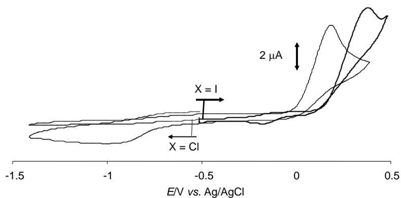
**Figure 3.** Cyclic voltammogram of compounds  $\text{MoOX}_2(\text{PMe}_3)_3$  in THF. Thinner curve:  $\text{X} = \text{Cl}$ ; thicker curve:  $\text{X} = \text{I}$ .  $C_{\text{Mo}} = 4 \cdot 10^{-3} \text{ M}$ . Scan rate =  $100 \text{ mV s}^{-1}$ .
