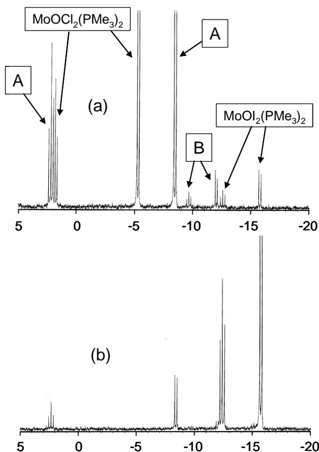
**Figure 4.** Room temperature  $^{31}\text{P}\{^1\text{H}\}$  NMR spectra of  $\text{MoOCl}_2(\text{PMe}_3)_3$  (50 mg, 0.12 mmol) and NaI in acetone- $d_6$  (0.6 mL). (a) After 5 h with 1 equiv NaI. (b) After 2.5 h from spectrum (a) with excess NaI.
