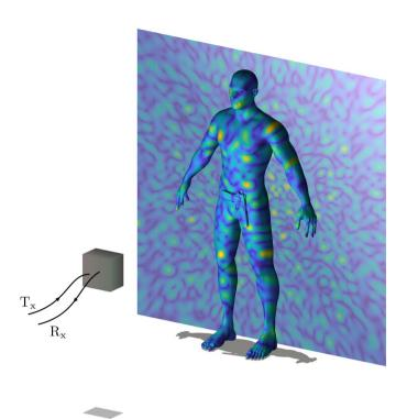
**Figure 1.** Illustration of a computational imaging system. The fields radiated in transmission and reception by a frequency diverse system interact with a target to be imaged. The scene  $\rho$  is interrogated by a succession of quasi-random field distributions varying according to the frequency and measurement ports. By means of simple frequency sweeps, spatial information is quickly encoded into a set of measurements gathered in  $\mathbf{g}$ .
