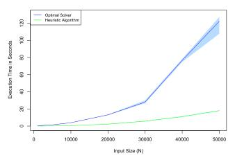
FIGURE 2. The average execution time of the optimal solution (blue curve) and the heuristic algorithm (green curve) with minimum and maximum values.
