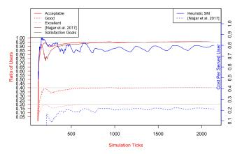
FIGURE 4. User acceptability rate (left y-axis) and its cost (right y-axis) using the proposed heuristic Satisfaction Management (SM) algorithm compared to [4].
