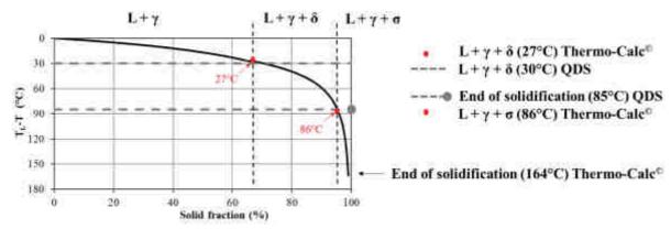
Figure 3 – Experimental and numerical solidification path
