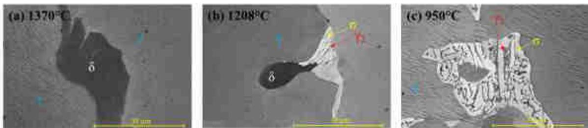
**Figure 2** – BSE micrographs of three different representative zones of the QDS sample : (a)  $1370^{\circ}\text{C} \pm 15^{\circ}\text{C}$ , in the mushy zone composed of austenite dendrites and  $\delta$ -ferrite, (b)  $1208^{\circ}\text{C} \pm 15^{\circ}\text{C}$ , partial eutectoid transformation of the  $\delta$ -ferrite into  $\sigma + \gamma_2$ , (c)  $950^{\circ}\text{C} \pm 15^{\circ}\text{C}$ ,  $\delta$ -ferrite is fully transformed into  $\sigma + \gamma_2$ .
