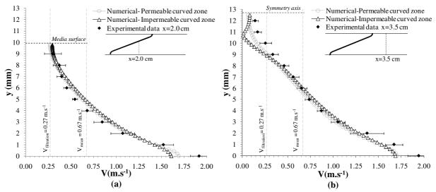
**Fig. 9.** Influence of pleat curved-zone permeability on numerical velocity profiles (calculated with the laminar airflow model) downstream of the filter for  $V_{mean} = 0.67 \text{ m.s}^{-1}$  ( $V_{filtration} = 0.27 \text{ m.s}^{-1}$ ): at (a) x = 2.0 cm; and at (b) x = 3.5 cm.
