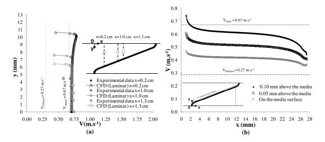
Fig. 10. (a) Numerical (calculated with the laminar airflow model) and experimental transversal velocity profiles upstream of the filter at x = 0.2 cm, x = 1.0 cm and x = 1.3 cm for V<sub>mean</sub> = 0.67 m.s<sup>-1</sup> (V<sub>filtration</sub> = 0.27 m.s<sup>-1</sup>).
