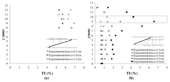
Fig. 11. Experimental transversal turbulence intensity profiles for  $V_{mean} = 0.67 \text{ m.s}^{-1}$  ( $V_{filtration} = 0.27 \text{ m.s}^{-1}$ ) (a) upstream of the filter at x = 0.2 cm, x = 1.0 cm and x = 1.3 cm; (b) downstream of the filter at x = 1.5 cm, x = 2.0 cm, x = 3.0 cm, x = 3.5 cm and x = 5.0 cm.
