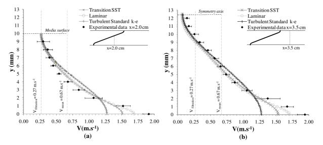
Fig. 8. Comparison of numerical and experimental transversal velocity profiles downstream of the filter for  $V_{mean} = 0.67 \text{ m.s}^{-1}$  ( $V_{filtration} = 0.27 \text{ m.s}^{-1}$ ): at (a) x = 2.0 cm; and at (b) x = 3.5 cm.
