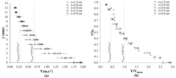
Fig. 7. Experimental transversal velocity profiles downstream of the filter for  $V_{mean} = 0.67 \text{ m.s}^{-1}$  ( $V_{filtration} = 0.27 \text{ m.s}^{-1}$ ).
