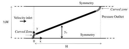
Fig. 3. Simulation domain and boundary conditions.
