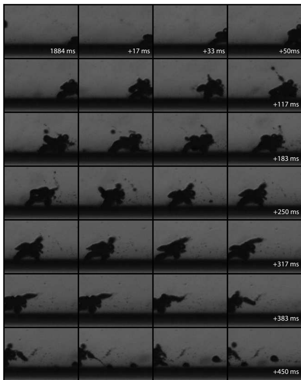
Figure 5: Morphing microfoam during sonication at 7 MHz and 86 kPa peak-negative pressure. The frame size corresponds to 274 \times 198 (\mu\text{m})^2 . Time t = 0 was defined by the start of the sonication.
