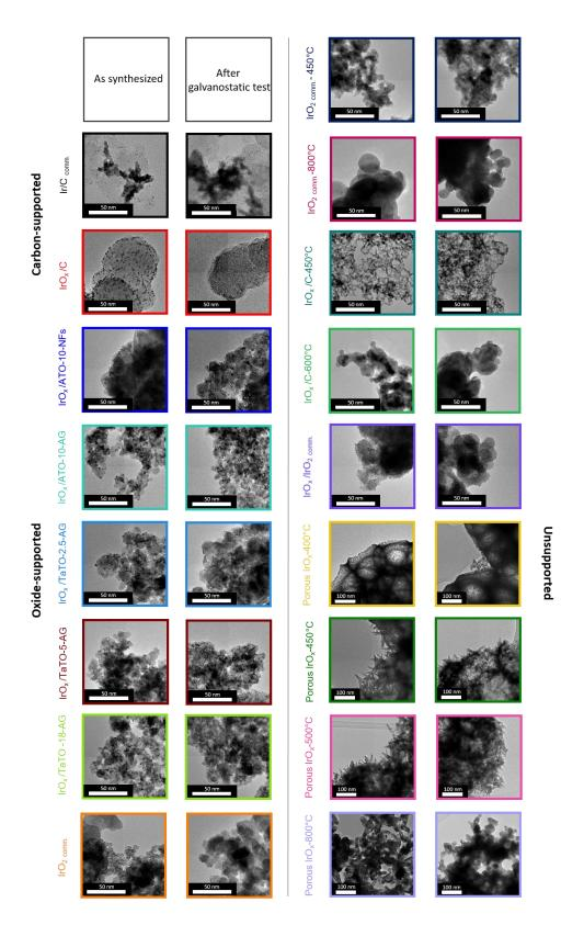
**Figure 3.** Transmission electron microscopy images of the electrocatalysts before/after the AST (Ar-saturated 0.05 M H<sub>2</sub>SO<sub>4</sub>, j = 10 mA cm<sup>-2</sup><sub>geo</sub>, T = 80 °C,  $U_{\text{cut-off}} = 2$  V vs. RHE).
