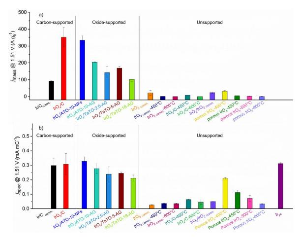
**Figure 2.** Initial (a) Ir mass-normalized and (b) charge-normalized OER activities measured at 1.51 V vs. RHE for the various catalysts used in this study. The charge in (b) was calculated by integration of the base voltammograms in the potential region 0.4 - 1.4 V vs. RHE (anodic potential sweep). All curves were recorded in 0.05 M  $H_2SO_4$  at T = 25 °C. The error bars correspond to the standard deviation calculated from at least two independent measurements.
