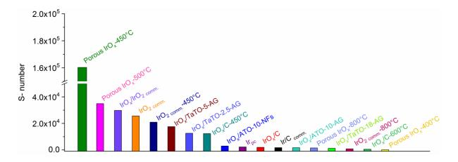
**Figure 5.** S-number values calculated for all the electrocatalysts during a galvanostatic AST performed in Ar-saturated 0.05 M H<sub>2</sub>SO<sub>4</sub> at j = 10 mA cm<sup>-2</sup>geo, T = 80 °C,  $U_{\text{cut-off}} = 2$  V vs. RHE.
