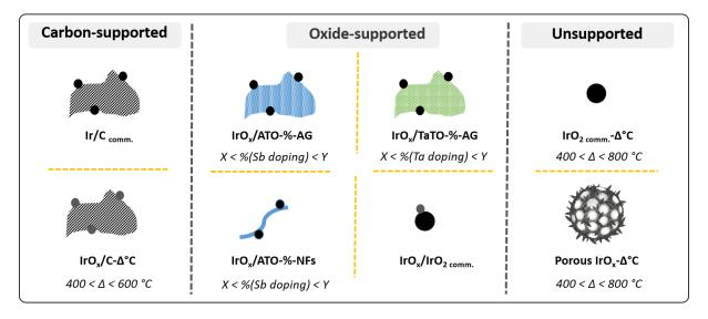
**Figure 1**. Scheme of the library of materials constituted to benchmark the OER activity and the stability of the different IrO<sub>x</sub> nano-/micro-particles. AG and NFs stand for aerogel and nanofibers, respectively.
