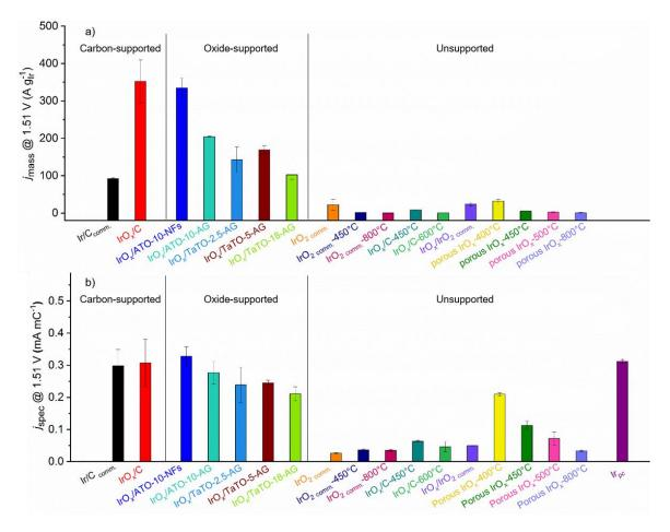
**Figure 2.** Initial (a) Ir mass-normalized and (b) charge-normalized OER activities measured at 1.51 V *vs*. RHE for the various catalysts used in this study. The charge in (b) was calculated by integration of the base voltammograms in the potential region 0.4 - 1.4 V *vs*. RHE (anodic potential sweep). All curves were recorded in 0.05 M H<sub>2</sub>SO<sub>4</sub> at T = 25 °C. The error bars correspond to the standard deviation calculated from at least two independent measurements.
