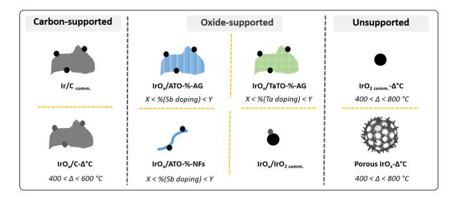
**Figure 1**. Scheme of the library of materials constituted to benchmark the OER activity and the stability of the different IrO<sub>x</sub> nano-/micro-particles. AG and NFs stand for aerogel and nanofibers, respectively.
