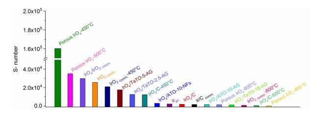
**Figure 5.** *S*-number values calculated for all the electrocatalysts during a galvanostatic AST performed in Ar-saturated 0.05 M H<sub>2</sub>SO<sub>4</sub> at j = 10 mA cm<sup>-2</sup><sub>geo</sub>, T = 80 °C,  $U_{\text{cut-off}} = 2$  V vs. RHE.
