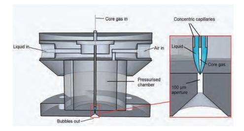
this flow exits the device alongside the surrounding air flow, the sharp pressure drop causes turbulent behaviour, breaking the core gas stream into microbubbles.
