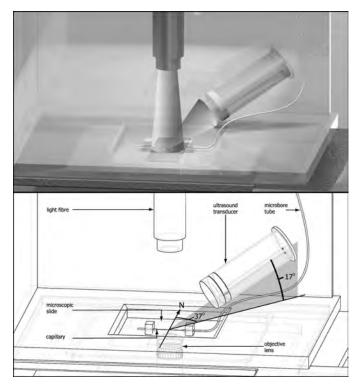
Figure 11 - Close-up of the sonication tank coinciding sound, light beam and objective focus (top) and definitions of the azimuth and elevation of the transducer relative to the North of the container (bottom).
