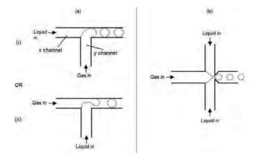
Figure 1 – (a) Possible T-junction microfluidic device configurations, (b) Flow-focusing device.
