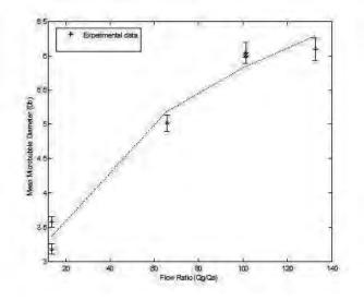
Figure 4 - graph showing flow ratio vs microbubble diameter.
