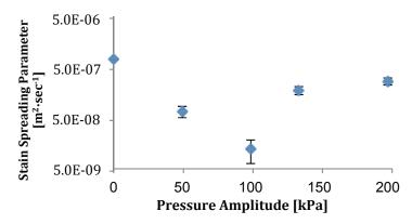
Figure 9 - Stain spreading parameter vs. various pressure amplitudes.
