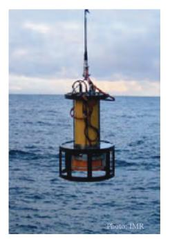
Figure 15 - TS Probe from IMR.
