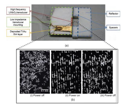
Figure 5 - (a) Manufactured and assembled prototype device, (b) 10  $\mu m$  polystyrene beads trapped in an ultrasonic standing wave field [8].
