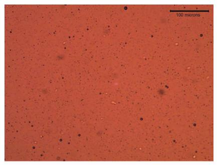
Figure 5 - Lipid-stabilised perfluorobutane bubbles. Scale bar represents 100  $\mu$ m.
