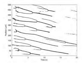
**Figure 14** - Cluster positions as a function of time, during continuous sonication at 7 MHz and 22kPa peak-negative acoustic pressure. Position in the capillary is defined from East (0  $\mu$ m) to West (500  $\mu$ m). Bold lines indicate merged clusters. The beginning (left) of a line indicates the formation of a cluster of diameter > 6.8  $\mu$ m. The end (right) of a line indicated the disintegration or contraction of a cluster to a diameter < 6.8  $\mu$ m.
