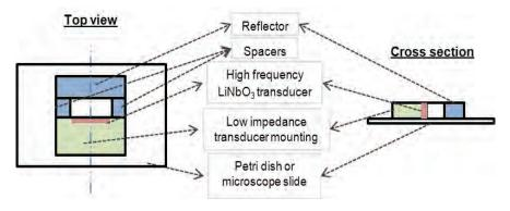
Figure 2 - Schematic of high frequency single element resonator
