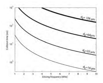
**Figure 9** – Collision times of individual encapsulated microbubbles as a function of driving frequency at given distances  $d_0$ , using  $p_a = 20$  kPa,  $R_0 = 1.25$  µm,  $\kappa = 5 \times 10^{-6}$  m<sup>2</sup> N<sup>-1</sup> and  $\rho = 998$  kg m<sup>-3</sup>.
