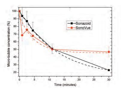
**Figure 3** - Concentration of two UCAs as a function of time in quiescent state, as measured by the spectrophotometer. Exponential decay curves (dashed) are fitted to each for comparison. Solutions were gently agitated before each measurement in order to counter any effects of buoyancy.
