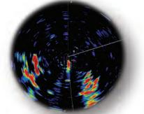
Figure 4 - A Simrad SP90 sonar showing shoa fish on both side of the ship.
