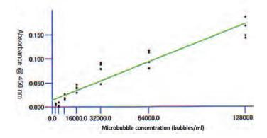
**Figure 1** - Calibration plot showing the absorbance (y-axis) versus microbubble concentration (x-axis), with each datum replicated 4 times and a linear plot of best fit established (with correlation coefficient = 0.973).
