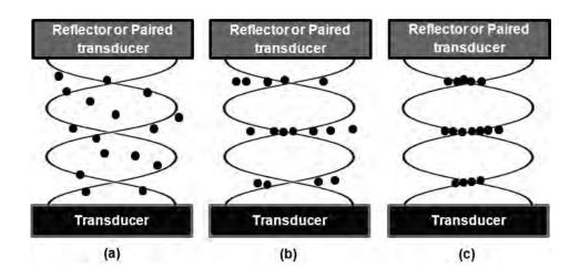
**Figure 1** - Particle motion within an ultrasonic standing wave [5]. (a) A standing wave is formed in a fluid, (b) particles move to pressure nodal planes due to the axial radiation force, (c) particles aggregate within the nodal planes because of the lateral radiation forces and Bjerknes forces.
