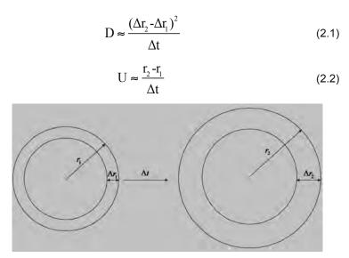
Figure 6 - Illustration of the dye spreading and approximated calculation of the parameters.
