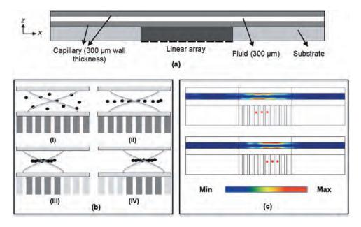
**Figure 7** - (a) Cross-section of 1D array manipulation device with capillary; (b) particle lateral manipulation with shifting active array elements; (c) Finite element simulation of shifting the position of potential energy density.
