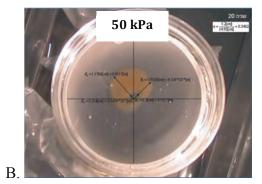
Figure 5 - Evaluating streaming and microstreaming in the plate above the cells. A) The apparatus that was used to estimate the generated streaming field in the US system; B) An example for the coffee stain dimensions.
