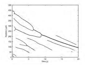
**Figure 13** - Cluster positions as a function of time, during continuous sonication at 2 MHz and 20kPa peak-negative acoustic pressure. Position in the capillary is defined from East (0  $\mu$ m) to West (500  $\mu$ m). Bold lines indicate merged clusters. The beginning (left) of a line indicates the formation of a cluster of diameter > 6.8  $\mu$ m. The end (right) of a line indicated the disintegration or contraction of a cluster to a diameter < 6.8  $\mu$ m.
