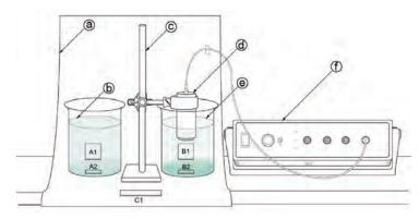
**Figure 3** – Experimental setup: (a) white paper sheet; (b) control sample; (c) clamp stand; (d) transducer; (e) sonicated sample; (f) pulser-receiver. Areas A1-B2 represent brightness measurement areas, C1 represents the calibration area.
