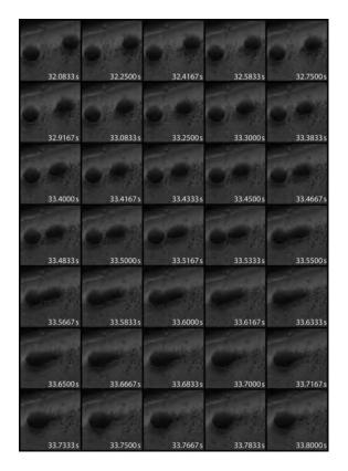
**Figure 15** – Two clusters, with 22-µm diameters and an initial distance of 55-µm, colliding and merging during continuous sonication at a 2-MHz driving frequency and a 20-kPa peak-negative pressure. The frame size corresponds to  $81 \times 81 \ (\mu m)^2$ . Times are relative to the start of the sonication (t = 0).
