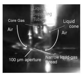
Figure 3 - Cone formation between capillaries and 100  $\mu m$  aperture (see also Fig.2 inset). Here the capillaries are slightly misaligned to the right of the aperture, hence the cone twists to the left to pass through.
