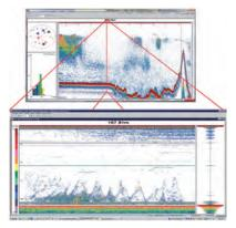
Figure 1 - Two approaches to the same area (Courtesy IMR). The two pictures are showing EK60 echograms from the same area from two different platforms. The upper echogram is recorded from a ship moving. Fish is detected in the water column above the seabed in the exact time when the ship was passing along a transect. The lower echogram shows behaviour of biomass in the exact point over time, recorded buy a acoustic buoy. This echogram shows the behaviour pattern of feeding saithe (Courtesy IMR).
