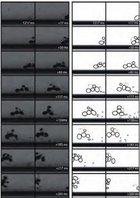
Figure 16 – Clusters forming during sonication at 7 MHz and 22-kPa peak negative pressure. The frame size corresponds to  $560 \times 264 \ (\mu m)^2$ . Time t = 0 was defined by the start of the sonication.
