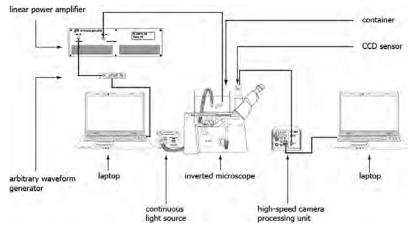
Figure 10 - Schematic overview of the experimental setup.
