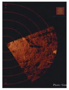
Figure 10 - Picture from a Simrad Mesote searchlight sonar.
