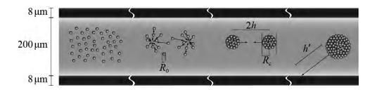
**Figure 19** – Schematic representation of the four stages of microfoam formation in a capillary: (leftright) random bubble distribution before ultrasound arrival, bubble colliding during sonication, cluster mergence within the space of a quarter of the wavelength, microfoam translation.
