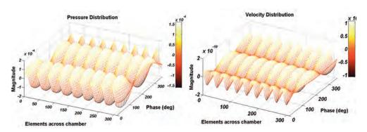
Figure 4 - Pressure (left) and velocity (right) distribution across water chamber with different phase.
