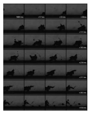
Figure 18 - Morphing microfoam during sonication at 7 MHz and 86 kPa peaknegative pressure and a schematic representation of the event. The frame size corresponds to  $274 \times 198 \ (\mu m)^2$ . Time t = 0 was defined by the start of the sonication.
