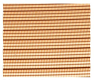
**Fig. 2.** Raw SPIRou spectrum of the FP étalon (zoom to the same central region as Fig. 1). Light from the lamp is being fed to both the science and calibration fibres. Around eight orders can be seen, centred around 1560 nm.
