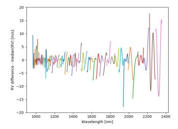
**Fig. 7.** Night-to-night variations of the FP wavelength solution: difference (in RV space) between the solutions generated with method FP2 for the 21 and 22 February 2019, using a fixed cavity width fit. The median value of the absolute RV differences is 0.8 m s<sup>-1</sup>. The drift induced by the fixed set of prior calibrations has been corrected.
