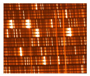
**Fig. 1.** Raw SPIRou spectrum of the UNe HC lamp (zoom to the central region). Light from the lamp is being fed to both the science and calibration fibres. Around eight orders can be seen, centred around 1560 nm. Three 'ghost' lines are also visible, corresponding to contamination from strongly saturated lines in other orders.
