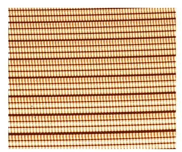
**Fig. 2.** Raw SPIRou spectrum of the FP étalon (zoom to the same central region as Fig. 1). Light from the lamp is being fed to both the science and calibration fibres. Around eight orders can be seen, centred around 1560 nm.
