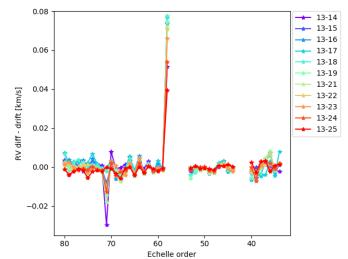
Fig. 9. Drift-corrected CCF RV differences per order for star A (left) and star B (right), using wavelength solutions from different nights. The strong variations of echelle order 58 for star B are due to a poor CCF fit.
