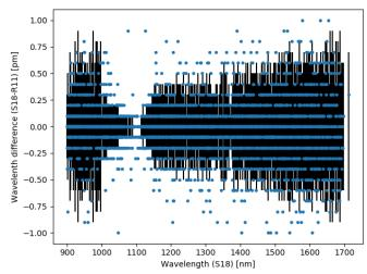
Fig. 3. Comparison of wavelengths for common lines between the catalogues of Redman et al. (2011) (R11) and Sarmiento et al. (2018) (S18). The blue points represent the difference in wavelengths, the black lines the S18 error bars. Points without error bars indicate that S18 reported no uncertainty for that line. The differences in wavelength are generally within the error bars when known, and always small.
