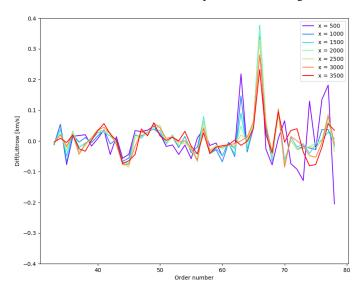
**Fig. 4.** Example Littrow solution check, showing the residuals of cross-order fits between the inverse echelle orders and the fractional wavelength contribution. Each line corresponds to a different pixel position. It should be noted that for the bluest orders, there is very little flux at pixels 500 and 3500.
