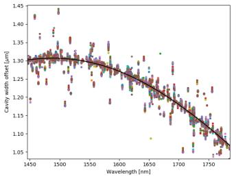
**Fig. 6.** Construction of a stable lines catalogue. Top: Overall cavity width fit (black line) from the HC lines (dots) for fifty exposures. Bottom: Zoom showing how the values for each line cluster together, but can be offset from the main fit. For scale, a cavity width offset of 0.2  $\mu$ m corresponds to a velocity offset of 4.88 km s<sup>-1</sup>, using the FP equation and the initial cavity width value of 2d = 24.4999 mm.
