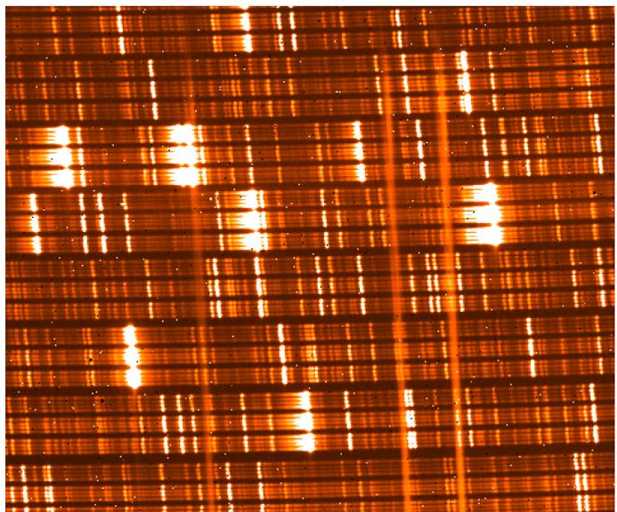
**Fig. 1.** Raw SPIRou spectrum of the UNe HC lamp (zoom to the central region). Light from the lamp is being fed to both the science and calibration fibres. Around eight orders can be seen, centred around 1560 nm. Three 'ghost' lines are also visible, corresponding to contamination from strongly saturated lines in other orders.
