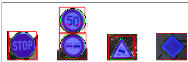
Fig. 6. Comparison with Mask R-CNN. In transparent blue, the mask predicted by Mask R-CNN, in green the shape predicted by our regression networks, and in black the ground truth annotated shape.
