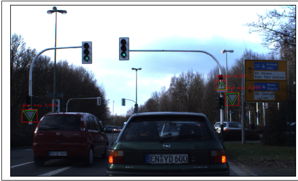
Fig. 4. Resulting image with boundaries drawn on the original image. Detection bounding boxes, classes and scores are represented in red. These boxes are cropped, resized and passed to the regression part to find vertices or ellipses and then resized back and drawn to the original image (in green). (best seen in color)
