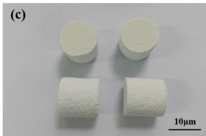
Fig. 9. Green bodies of Al 2 O 3 PHM Ceramics, before debinding process [113]. (For interpretation of the references to color in this figure legend, the reader is referred to the Web version of this article.)
