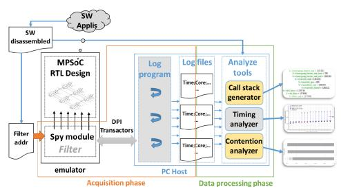
Fig. 2. Diagram of implementation of our non-intrusive tool chain measurement with MPSoC systems.
