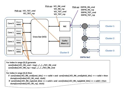
Fig. 8. Illustration of signals dumping for contention analysis.
