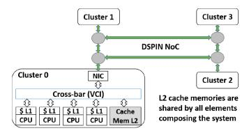
Fig. 5. 4-cluster (16-core) TSAR MPSoC architecture.
