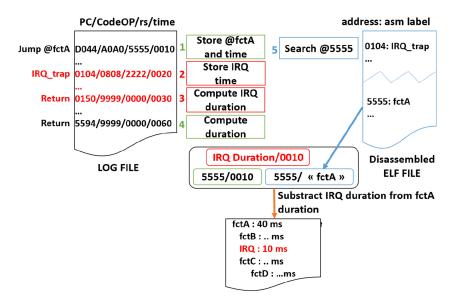
Fig. 4. Call stack generator working example.
