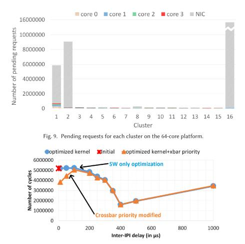
Fig. 10. Full release time of 64 threads according to the delay introduced between two send of IPI with the modification of the crossbar priority.
