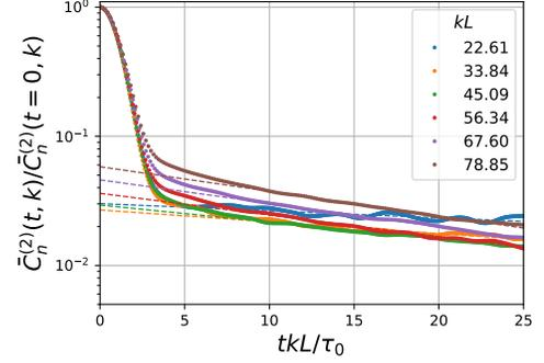
FIG. 10. Time dependence of the normalized two-point correlation function of the velocity norms  $\bar{C}_n^{(2)}(t, k)$  at  $R_\lambda = 60$  for different wavenumbers  $k$  in semi-logarithmic scales. The numerical data are denoted with dots, the exponential fit is denoted with the dashed lines.
