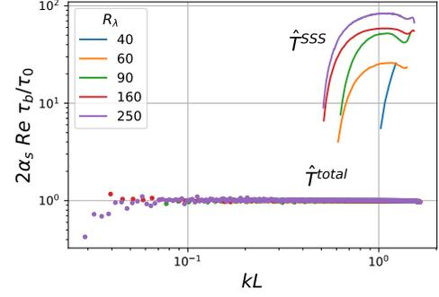
FIG. 9. Dependence of the parameter  $\tau_b$  of the fitting function Eq. (29) on the wavenumber for the small scale advection-velocity correlation  $\hat{T}^{SSS}$  (continuous) and for the total one  $\hat{T}$  (dotted lines). The values are normalized by  $2\alpha_S Re / \tau_0$  to enable comparison with the Eq. (25).
