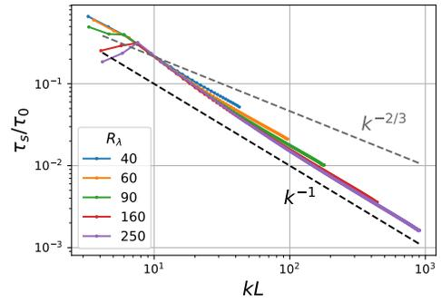
FIG. 3. Dependence of the decorrelation time  $\tau_s$  resulting from the Gaussian fit on the wavenumber in log-log scale for various  $R_\lambda$ . Times on the vertical axis are normalized by the large eddy turnover time scale  $\tau_0$ , the wavenumber on the horizontal axis is normalized by the integral length scale  $L$ .
