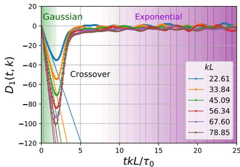
FIG. 11. The normalized time derivative  $D_1$  defined in Eq. (32) calculated numerically with the data from the simulation at  $R_\lambda = 60$ . The linear part of  $D_1$ , highlighted by green shades, corresponds to the Gaussian decay at small time delays, and the approximately constant part of  $D_1$ , highlighted by purple shades, corresponds to the exponential time correlation at large time delays.
