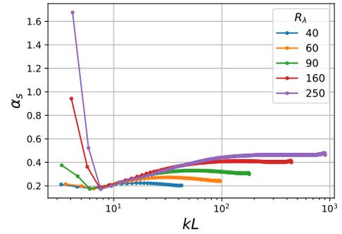
FIG. 4. Estimation of the theoretical parameter  $\alpha_S$  in the Eq. (2) from the results of the fit of numerical data.
