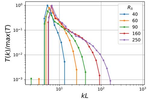
FIG. 5. Rate of the direct energy transfer from the forcing range to the wavenumber  $k$  normalized by the maximal value at various Reynolds numbers computed with the use of the shell-to-shell energy transfer method described in Ref. 41.
