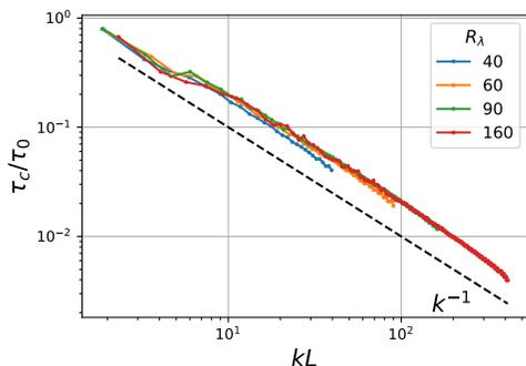
FIG. 12. Crossover time for the two-point correlations of the velocity norms  $\bar{C}_n^{(2)}$  between the small time and large time regimes as a function of the wavenumber  $k$ , estimated from the minimum of  $D_1$ .
