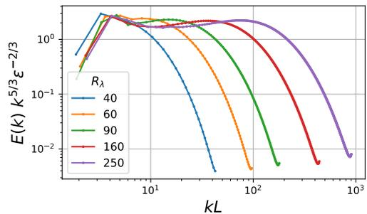
FIG. 1. Compensated spatial spectrum of the kinetic energy obtained from the averaged two-point spatio-temporal correlation function  $C^{(2)}$  at zero time delay according to Eq. (19).  $\epsilon$  is the energy dissipation rate,  $L$  the integral length scale, and  $R_\lambda$  the Reynolds number at the Taylor microscale.
