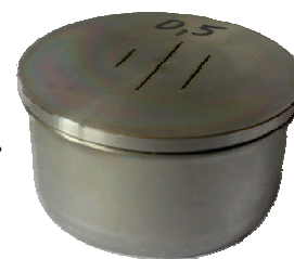
Figure 7. Process challenging device: 3 metal boxes with each 3 slits (0,3 mm, 0,5 mm and 0,7 mm)
