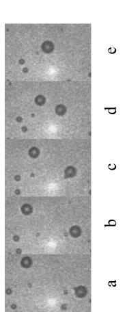
Figure 8: The approach of two  $\oslash 4\,\mu\mathrm{m}$  experimental UCA bubbles induced by a secondary radiation force. Each image frame corresponds to a  $30 \times 20\,\mu\mathrm{m}^2$  area. Frames are each captured after insonification by 10 cycles of  $0.5\,\mathrm{MHz}$  ultrasound (MI = 0.67).
