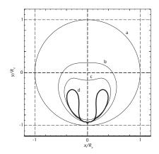
Figure 1: Schematic evolution of jet development in a collapsing bubble near a boundary (below): bubble on the verge of collapse (a), asymmetric collapse (b), jet development (c), funnel-shaped protrusion (d).
