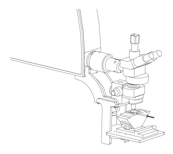
Figure 4: Line drawing of the optical observation part of the Brandaris-128 system.
