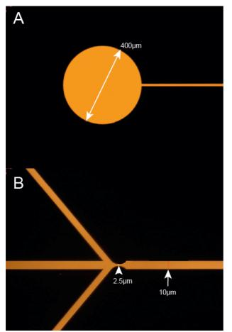
Figure 2: Result of e-beam lithography for a prototype microfluidic design. Image captured using optical microscopy. Panel A shows a disc that will be used as the input channel for the shell material or gas. Panel B shows a 2.5µm constriction in the region where the gas and lipid components meet.
