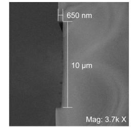
Figure 3: Result of plasma etching using  $CF_4$  gas for a total duration of 10 min. Image captured electron microscopy (e Line). A channel depth of 650nm was measured.
