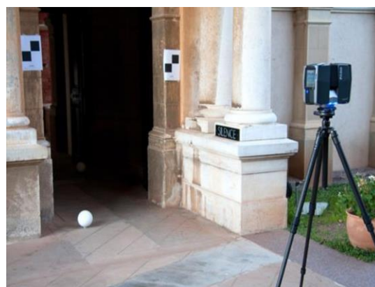
Figure 2: positioning station of the Faro Focus scanner, positioning the spherical targets and the black and white plane target to ensure the 3D survey, the registration and georeferencing - St Honorat, Lerins Monastery (FRANCE) - S. Sorin/CEPAM
