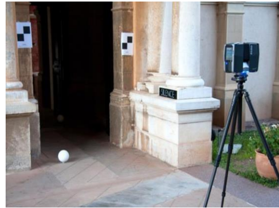
Figure 2: positioning station of the Faro Focus scanner, positioning the spherical targets and the black and white plane target to ensure the 3D survey, the registration and georeferencing - St Honorat, Lerins Monastery (FRANCE) - S. Sorin/CEPAM
