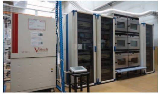
Fig. 7. The experimental setup for accelerated aging tests, climatic chambers and power electronic
