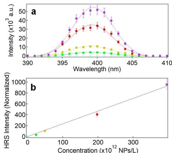
**Figure 5.** (a) Spectral response around 400 nm of the HRS intensities of LN NPs dispersions upon excitation with a vertically polarized wavelength at 800 nm. The corresponding NP concentrations are indicated in the lower panel whereas light blue dots stand for the spectral response of pure water. (b) Graphical plot of the normalized HRS intensities as a function of the NP concentration.
