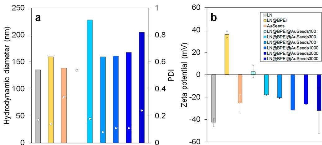
**Figure 4.** (a) Hydrodynamic diameters and PDI ( $\diamond$  symbol, shown on the corresponding hydrodynamic diameter bars) values for LN, LN@BPEI, AuSeeds and LN@BPEI@AuSeeds NPs. The hydrodynamic diameter value obtained for sample LN@BPEI@AuSeeds100 was larger than 1000 nm due to a significant agglomeration and was thus omitted from the graph. (b) Zeta potential values for LN, LN@BPEI, AuSeeds and LN@BPEI@AuSeeds NPs.
