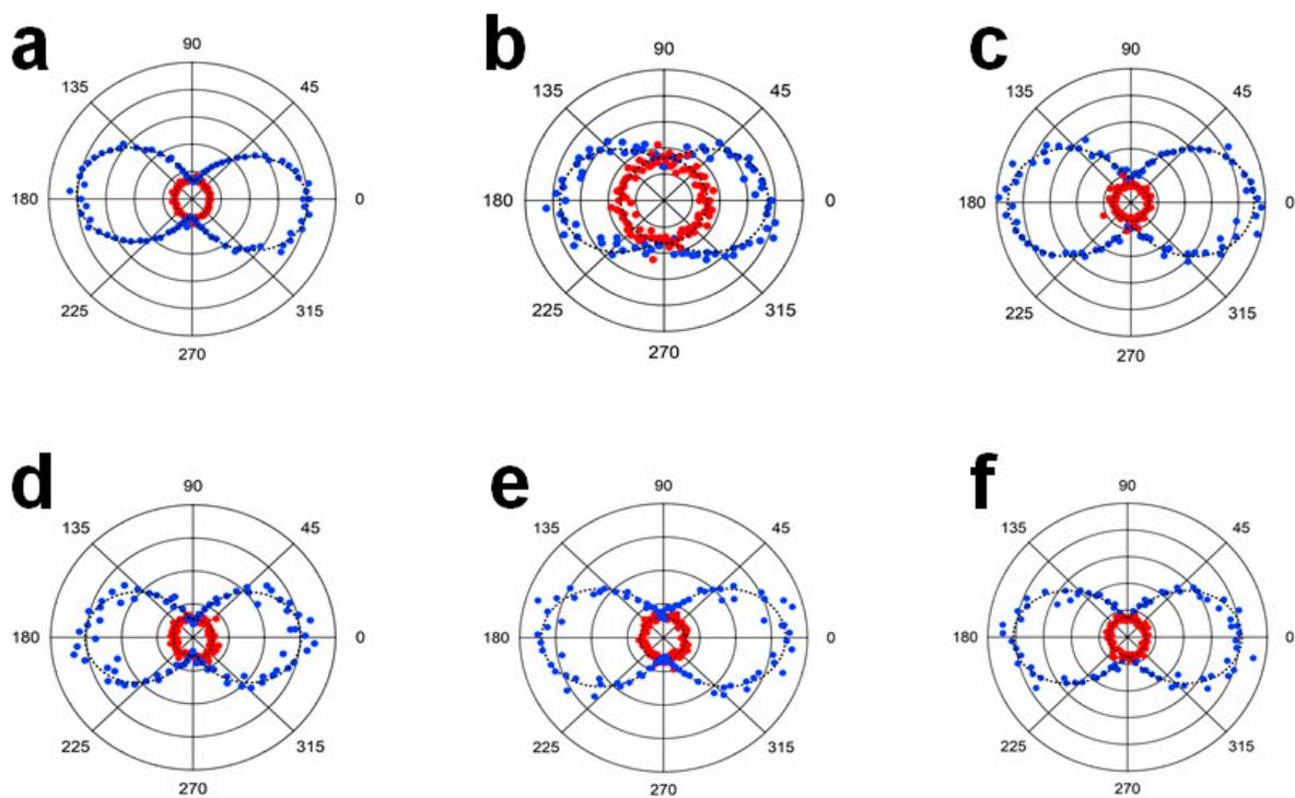
**Figure 7.** Polar plots of HRS intensities as a function of the polarization angles of the incident light. The blue and red data points correspond to vertical and horizontal harmonic polarization of the HRS intensities, respectively. (a) Core LN, (b) AuSeeds, (c) LN@BPEI@AuSeeds100, (d) LN@BPEI@AuSeeds300, (e) LN@BPEI@AuSeeds1000 and (f) LN@BPEI@AuSeeds3000.
