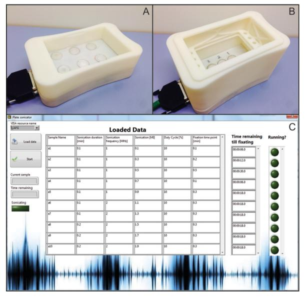
Figure 9 Completed devices and software. Photograph of the completed 24-well plate sonicator (A) and OptiCell<sup>™</sup> (B). (C) Screen capture of the user software interface.
