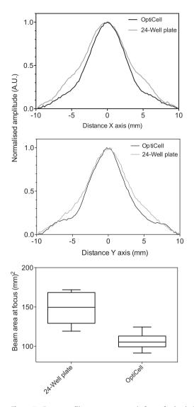
**Figure 7** Beam profile scans at acoustic focus for both devices (A and B) and whisker plot of the focal area for the two devices using a -3-dB cutoff. A statistically significantly smaller beam area is evident in the OptiCell<sup>™</sup> sonicator, due to the close proximity of the transducers (cf. Figure 6).
