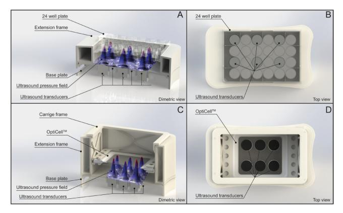
Figure 1 Computer generated renderings of prototype devices. Cutaway diagram showing assembly of ultrasound sonicators for 24-well plates (A and B) and OptiCells<sup>™</sup> (C and D) including the acoustic pressure fields. (B and D) Top view and position of the ultrasound transducers for both devices. In the OptiCell<sup>™</sup> sonicator, the ultrasound transducers have been places substantially closer.
