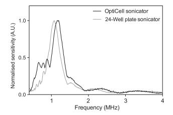
**Figure 5** Frequency sensitivity of sonicators. Peak sensitivity can be seen at 1.08 and 1.17 MHz for the 24-well plate and OptiCell<sup>™</sup> sonicator, respectively. Increased sensitivity is evident between 0.6 and 0.8 MHz in the OptiCell<sup>™</sup> sonicator. This directly correlates to the reflection coefficient magnitude shown in Figure 4.
