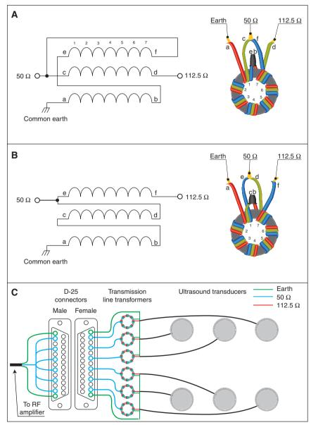
**Figure 3** Electrical impedance matching and connection diagrams. Transmission line transformers used to match 112.5- $\Omega$  transducers to 50  $\Omega$  (A and B). Both variation result in the same impedance ratio and can be used interchangeably. Wiring schematic from transducers to amplifier (C) showing the independent connection of each transducer in the case. All transducers can be driven simultaneously via an interconnected male connector.
