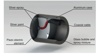
**Figure 2** Cutaway diagram showing components and assembly of the ultrasound transducers. The front face of the transducer has been connected to the earth via the case. This ensures a smooth front surface with no electrodes. A low-density glass bubble and epoxy mixture has been used as backing to support the piezo element with minimal damping.
