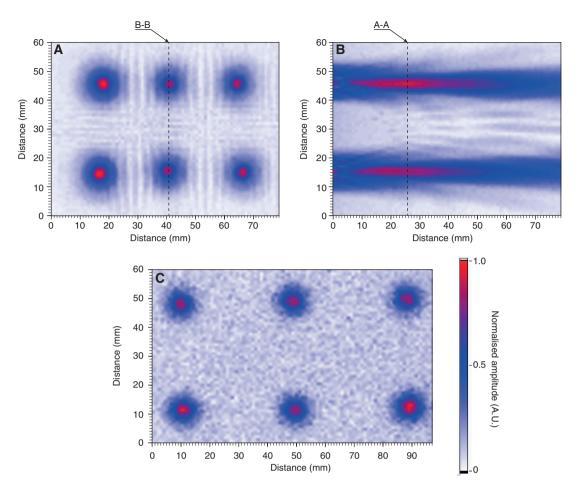
Figure 6 Field scans of plate sonicators. Scans A and B are the *xy* and *xz* scans of the OptiCell<sup>™</sup> sonicator. Line B-B indicates the location of scan B, wheras line A-A indicates the location of scan A. Scan C is the is the *xy* scan of the 24-well plate sonicator. All scans are at the same scale. Minor side lobes are evident in the OptiCell<sup>™</sup> sonicator due to the close proximity of the transducers. This was not seen in the 24-well plate sonicator.
