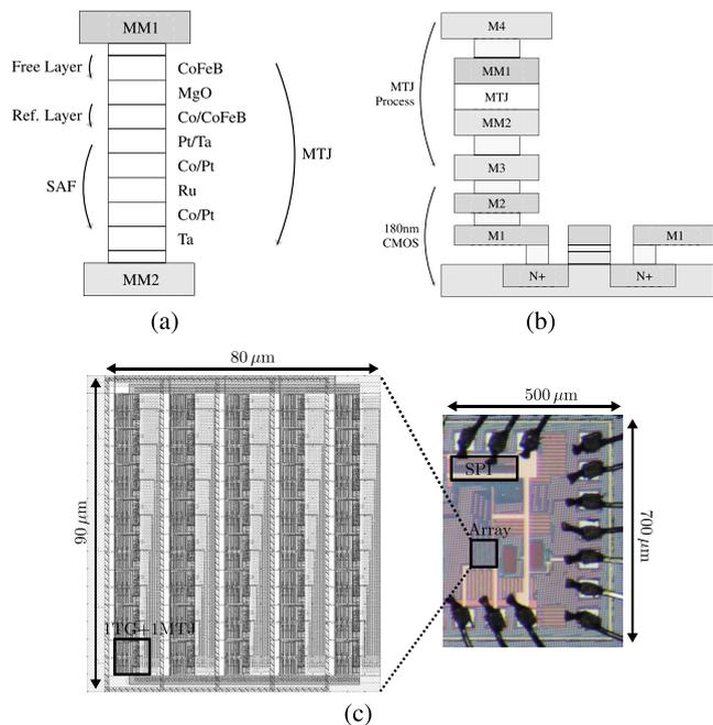
**Fig 2** (a) Layer composition of a perpendicular MTJ nanopillar. Thickness of each layer of the MTJ is as follows (in nm): MgO, FeCoB(0.5), MgO, FeCoB(1), Co(0.9), Pt(0.2), Ta(0.15),  $3 \times [0.5 \text{ Co}/0.2 \text{ Pt}]$ , Ru(0.8),  $6 \times [0.5 \text{ Co}/0.2 \text{ Pt}]$ (6). (b) Layer composition of the hybrid CMOS–MTJ technology. (c) Layout of the MTJ array and photograph of the MTJ array prototype chip
