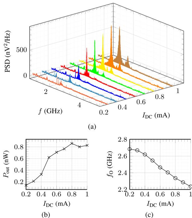
**Fig 4** (a) Measured output frequency spectra in dependence of  $I_{DC}$  for  $H = 1 \text{ kOe}$ . (b) Measured MTJ-based STO's output power  $P_{out}$  and (c) centre oscillation frequency  $f_0$  in dependence of injected DC current  $I_{DC}$
