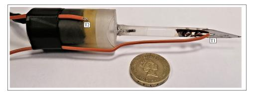
Figure 3: Position of the temperature probes on the ultrasonic knife on the blade (T1) and over the ultrasound transducer (T2).
