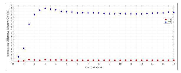
Figure 5: Temperature difference over a 15 minute period with the ultrasonic knife under sonication. The red dots indicate the temperature difference at the blade (T1) and blue diamonds indicate the temperature difference over the ultrasound transducer (T2).
