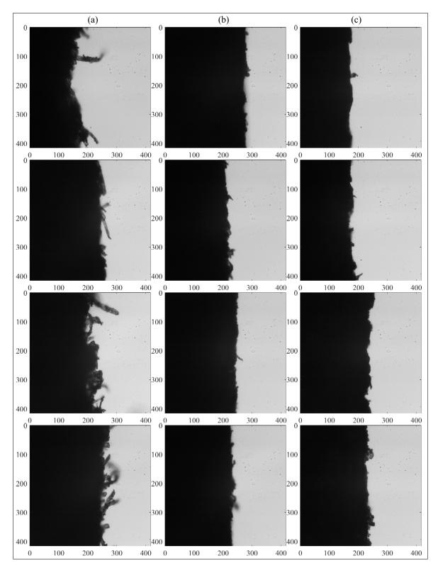
Figure 6: Back-lit bright-field  $10 \times$  microscopy images of incisions in paper from an unsonicated blunt blade (a) and a sonicated blunt blade (b), compared to the paper edge from sharp industrial cutting (c). The darks areas represent the paper. Each frame corresponds to a  $416 \times 416 \,(\mu m^2)$  area.
