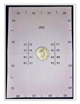
Figure 4: A6-sized experimental sheet with marks indicating the industrially cut edge (E1-E8) and along the incisions (F1-F8).
