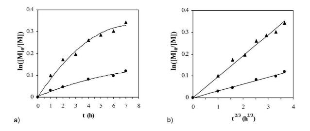
Figure 8. a) First and b) 2/3-order dependence of  $\ln[M]_0/[M]$  on time for the VAc polymerization initiated by the pink compound 2 with ( $\blacktriangle$ ) and without ( $\bullet$ ) pyridine (Table 3 and entry 2 of Table 1, respectively).
