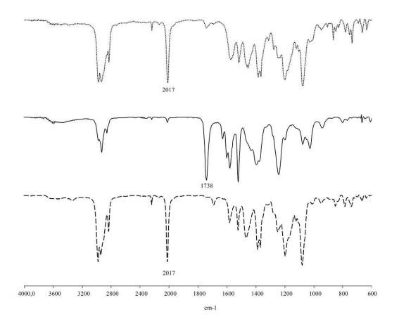
Figure 1. Infra-red spectra of green cobalt adduct  $1 (\dots)$  and pink cobalt adduct 2 (--) collected when reaction between V-70 and Co(acac)<sub>2</sub> was carried out in the presence of VAc. IR spectrum of green cobalt adduct 1 formed by reaction of V-70 and Co(acac)<sub>2</sub> without VAc (----). The cobalt adducts were dissolved in CH<sub>2</sub>Cl<sub>2</sub> and solvent-cast on a NaCl disk before IR analysis.
