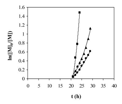
Figure 13. Plot of  $\ln([M]_0/[M])$  versus time for the vinyl acetate polymerization in the presence of  $Co(acac)_2$  at 30°C. Conditions : 21h of pre-reaction  $[VAc]/[Co(acac)_2]/[V-70] = 540/1/3$  then (•) no water added ( $\blacktriangle$ ) water saturated VAc ( $\blacksquare$ ) biphasic system :  $V_{VAc}/V_{H20.} = 4$ .
