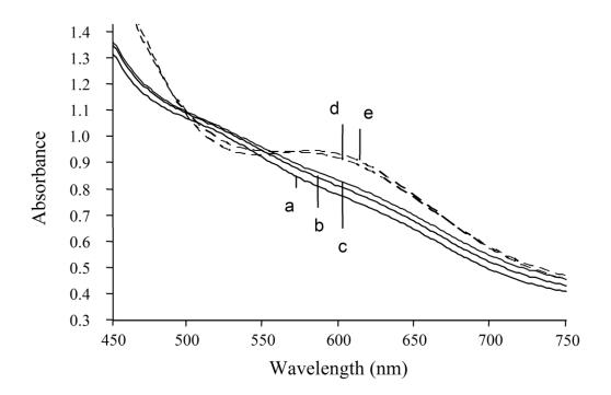
Figure 6. Evolution of the UV-visible spectrum of the pink cobalt adduct **2** in a degassed acetone/water mixture (9.5/0.5) (full lines) (a) t = 0, (b) t = 20 min, (c) t = 40 min under inert atmosphere, before exposure to air for 4 min between each scan (dotted lines) at (d) t = 60 min, (e) t = 100 min.
