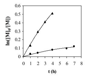
Figure 7. Time dependence of  $\ln[M]_0/[M]$  for the VAc polymerization initiated by the green compound  $1(\blacktriangle)$  and the pink compound  $2(\bullet)$ . (Table 1, entries 1 and 2, respectively)
