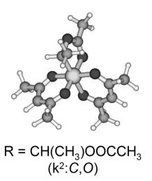
Figure 15. DFT optimized geometries of the model compounds R-Co(acac)<sub>2</sub>.
