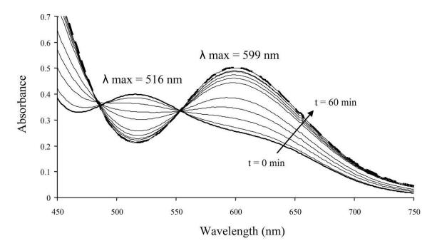
Figure 5. Evolution of the UV-visible spectrum of the pink compound **2** (broad full line,  $\lambda_{max} = 516$  nm) in degassed CH<sub>2</sub>Cl<sub>2</sub> when exposed to air. Spectra were collected every 5 minutes for 60 minutes until the color turned green (compound **3**, broad dotted line,  $\lambda_{max} = 599$  nm).
