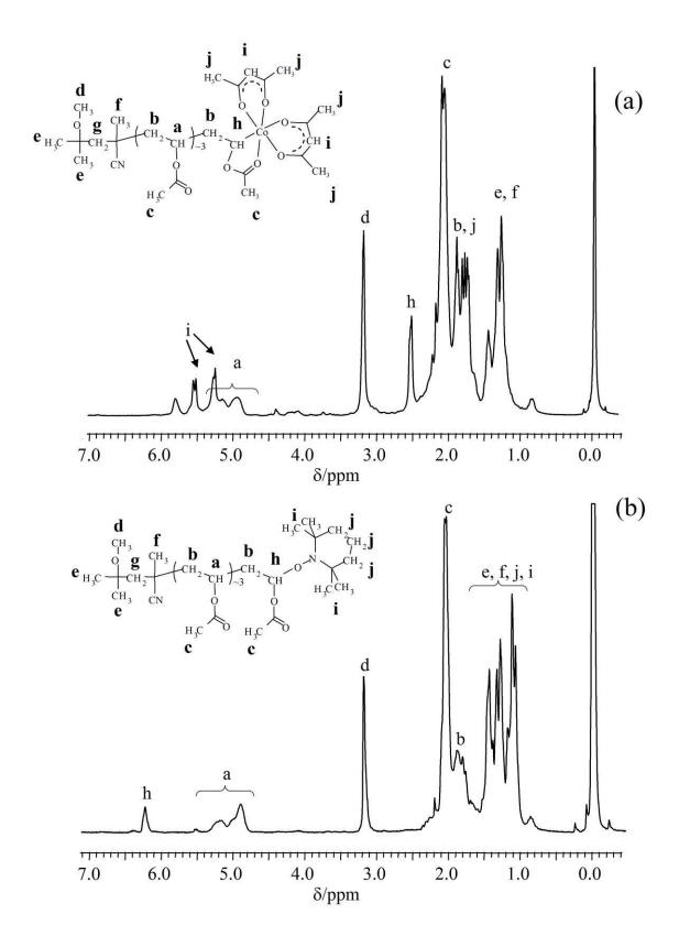
Figure 3. <sup>1</sup>H NMR spectrum for the low molecular weight cobalt adduct (2): (a) untreated; (b) after treatment with TEMPO (2'). Solvent =  $CDCl_3$ .
