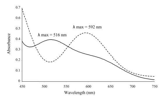
Figure 4. UV-visible spectra for the green compound 1 (dotted line,  $\lambda_{max} = 592$  nm) and the pink compound 2 (full line,  $\lambda_{max} = 516$  nm and 613 nm) in degassed CH<sub>2</sub>Cl<sub>2</sub>.
