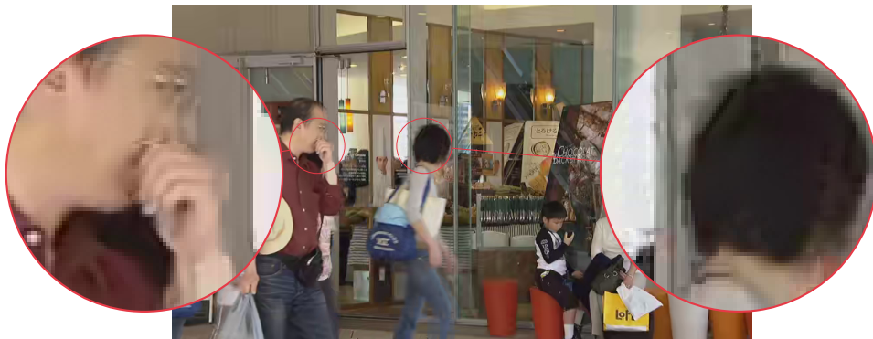
(b) HEVC: The PSNR of the GOP is 33.37 dB and the GOP rate is 1.42 Mbit/s.
