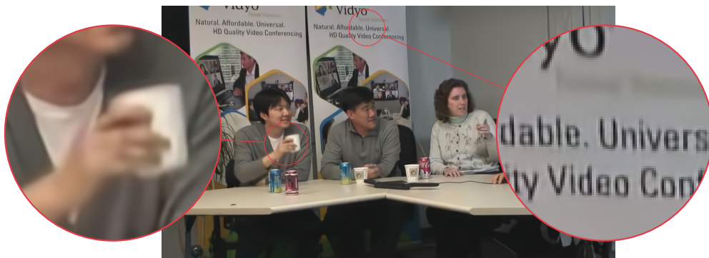
(c) Proposed system: PSNR of the GOP is 37.29 dB and the GOP rate is 1.21 Mbit/s.
