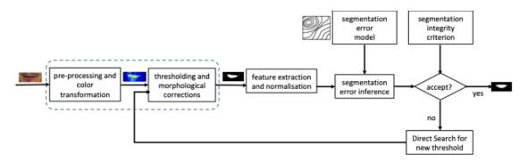
Fig. 2 Algorithm stage 2: Adaptive thresholding.
