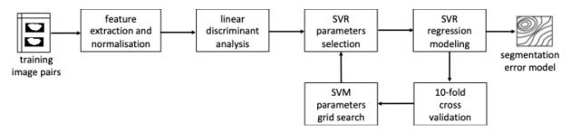
Fig. 1 Algorithm stage 1: Training of the segmentation error model.
