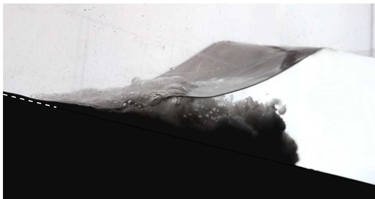
Figure 1. Oblique view of a particle-driven gravity current, generated by a gas-fluidized granular flow down an inclined plane entering water. The dashed line indicates the bottom of the inclined plane above the level of the undisturbed water surface. On the left, the subaerial granular flow is relatively thin, dense and rapid before evolving to a thick and dilute particle-driven gravity current underwater. An impulse wave is also generated on the water surface, which has already been studied in Bougouin et al. (2020).
