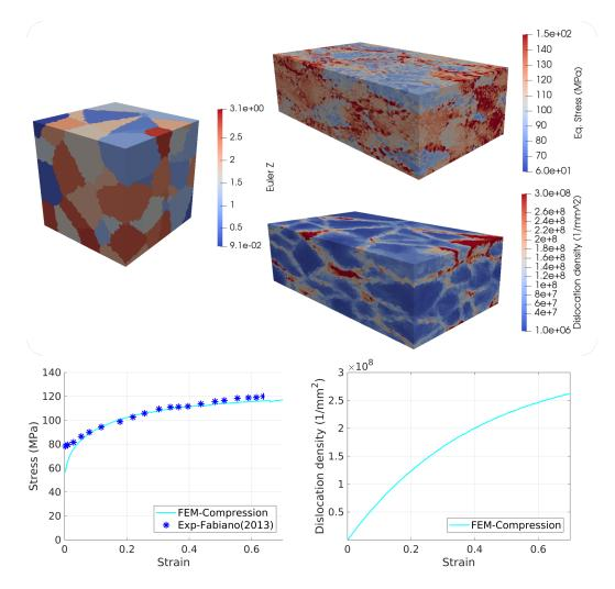
Figure 9: Channel die compression, in terms of average stress and average dislocation density, of a 304L 0.5 \* 0.5 \* 0.5 mm - 100 grains polycrystal. The experimental data from Fabiano [64] was obtained by digitalizing the published data.
