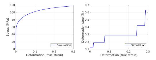
Figure 14: Stress vs strain curve (left side) and Deformation step vs strain curve (right side) for CP simulation of 304L steel at a constant strain rate of  $0.01s^{-1}$ .
