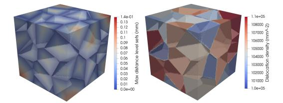
Figure 1: Max value of LS functions (left side) and initial dislocation density constant per grain (right side) in an unstructured finite element mesh representing 3D microstructure generated using Voronoi tessellation. Contours show the 0 value of the level set functions, i.e. the grain boundary network.
