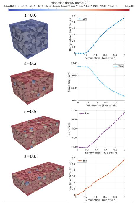
Figure 5: Example simulation of compression of a domain composed of 400 initial grains.
