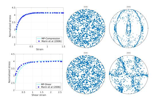
Figure 8: MP simulations of the deformation of an aggregate of 256 FCC crystals subjected to plane strain compression (top side) and to simple shear(bottom side). Macroscopic stress response (left side) and  $\langle 111 \rangle$  pole figures before deformation (center) and after deformation (right side). The data from Marin [54] was obtained by digitalizing the published data.
