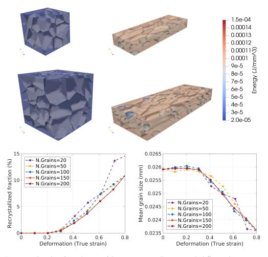
Figure 16: Results of simulations of dynamic recrystallization with different domains sizes, ranging from 20 to 100 initial grains, in terms of X (left) and  $\overline{R}$  (right).
