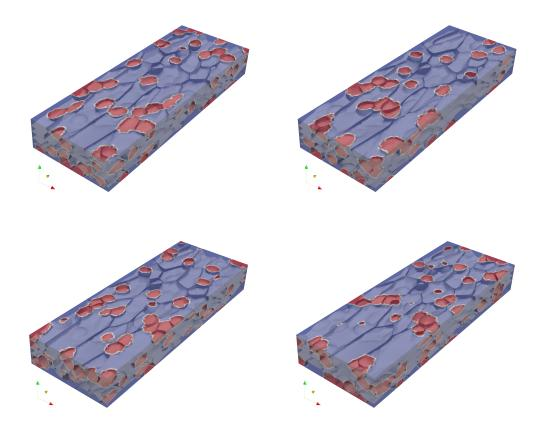
Figure 21: Recrystallized grains of simulations with different criteria for nucleus position. Top left case 1, top right case 2, bottom left case 3 and bottom right case 4. Red color corresponds to the recrystallized grains.
