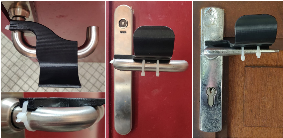
Fig. 5. Hands-free door openers using cable ties on two types of door handles.
