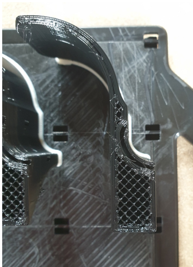
Fig. 3. Printing characteristics on a J120 device: layer thickness = 0.33 mm, filling density = 43%, wall thickness = 2 mm; the use of support was optimised in order to decrease post-treatment time.
