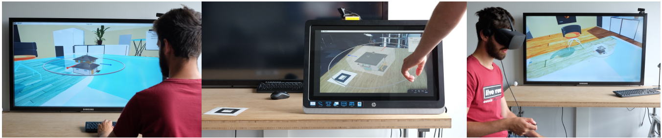
Figure 1: We propose a new model for designing VR, AR and MR applications independently of any device. Our model allows the user to visualize a virtual world and to interact with it on any kind of device. These pictures shows a user interacting with the same virtual object on a desktop, on a touchscreen and on an Oculus Rift HMD.
